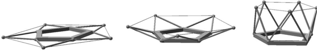
**Fig. 4.8:** Post-packed phenomenon: flipping up the bracings
