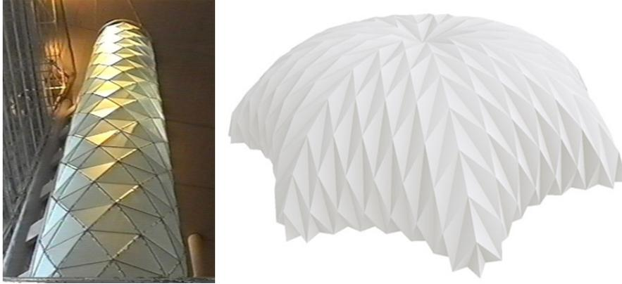
**Fig. 2.11:** Foldable tube (exhibition object) and dome (paper model) with the Yoshimura pattern [Yoshimura]
