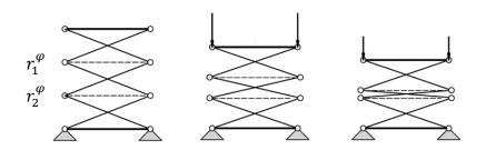
**Fig. 3.24:** Packing sequence without intermediate stiffening for k=3
