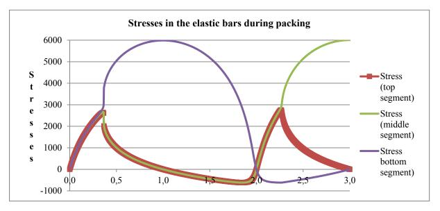
**Fig. 4.29:** Perturbation-controlled unrestricted simulation of packing a three-storey pentagonal mast — stresses in the elastic bars during packing
