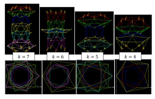
Fig. 4.47: Stochastic packing pattern of non-stiffened antiprismatic mast
