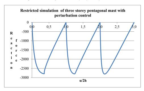
**Fig. 4.31:** Force-displacement diagram of three-storey pentagonal mast — perturbation controlled restricted simulation
