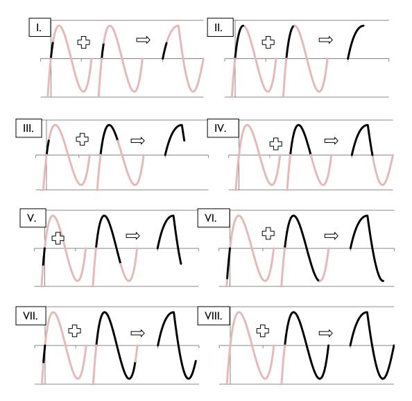
**Fig. 3.13:** Constructing the force-displacement diagram of deployable mast of two segments from the individual diagrams of separated segments without preventing 'post-packed phenomena' (see the packing sequence with the assigned configurations on Fig. 3.12,  $h_0/r_0=1$ )
