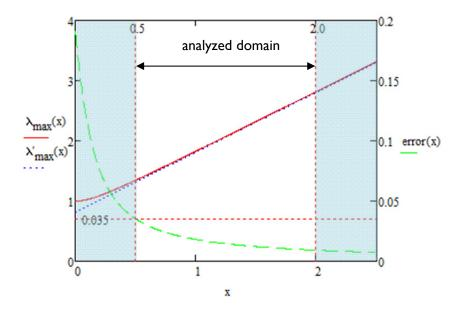
**Fig. 4.4:** Linear approximation for final stretching of elastic bars ( $\lambda$ ` $_{max} = \hat{\lambda}_{max}$ ) of pentagonal (n=5) antiprismatic unit in function of the height-radius ratio (x=h/R) (exact function (4.9) with continuous line ( $\lambda$ \* $_{max}(x)$ ), approximation of stretching (4.11) with dotted line ( $\lambda$ \* $_{max}(x)$ ), error of the approximation with dashed line)
