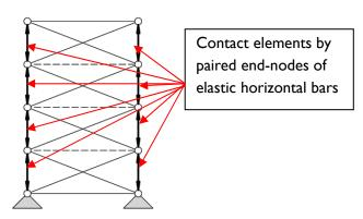
Fig. 3.56: Modeling the restriction of 'post-packed phenomenon' for non-stiffened masts
