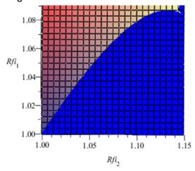
**Fig. 3.26:** The equilibrium path in the parameter field for k=4 (h/ro=1)
