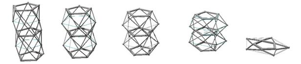
Fig. 4.17: Uniform restricted packing of antiprismatic deployable mast of two segments
