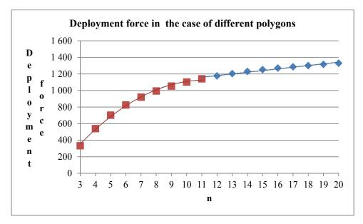
**Fig. 4.23:** Influence of geometrical configuration — deployment force (maximal reaction force multiplied by the number of vertices) of basic unit in case of different n-gons (EA = 500; h = 0.5; R = 0.5)
