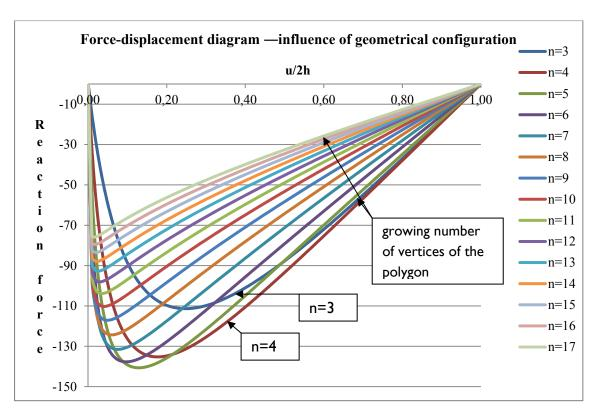
**Fig. 4.22:** Force-displacement diagram of basic unit in the case of different n-gons (EA = 500; h = 0.5; R = 0.5)
