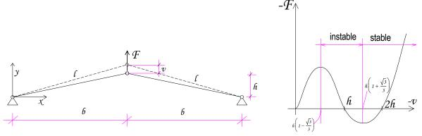
Fig. B1: shallow truss and its force-displacement diagram
