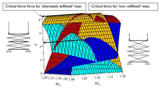
**Fig. 3.29:** Comparing critical forces of 'alternately stiffened' and 'non-stiffened' structures by plotting equilibrium paths in function of the half-lengths of the elastic horizontal bars (The equilibrium path of the 'alternately stiffened' mast is at the intersection of the light blue and the dark blue surfaces, the one of the 'non-stiffened' structure is at the intersection of the orange and red surfaces, EA=100,  $h_0=1$ ,  $r_0=1$ , initial total height of the structure:  $H=4h_0$ )
