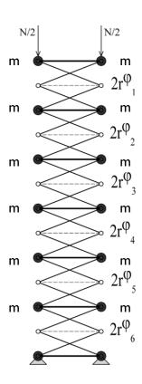
Fig. 3.16: Planar deployable mast with self-weight
