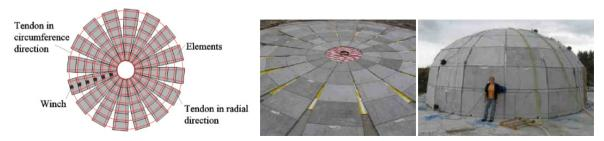
**Fig. 2.53:** Transformation of precast divided planar segments into a hemispherical dome [Dallinger and Kolleger, 2009]
