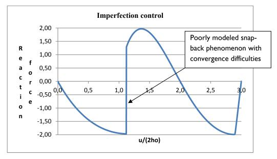
**Fig. 3.35:** Typical packing simulation of a three-storey planar mast without the restriction of 'post-packed phenomenon' controlled by the imperfection of axial stiffness values, downwards forces are negative  $(EA_1 = 100, EA_2 = 99.8, EA_3 = 99.6, h = 1, r_0 = 1)$
