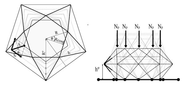
Fig. 4.6: Equilibrium of basic deployable unit
