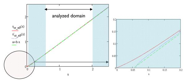
**Fig. 4.11:** Approximation of critical height: critical height/critical radius  $(x_{cr} = h_{cr}/R)$  in function of initial height/initial radius (x = h/R), for 9-gonal segment — exact solution with continuous line, approximation in accordance with (4.22) with dotted line, approximation in accordance with (4.23) with dashed line
