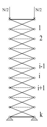
Fig. 3.20: Planar deployable mast without intermediate stiffening
