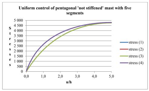
**Fig. 4.42:** Packing of pentagonal, non-stiffened mast of five segments (lb=lnec), packing sequence in Fig. 4.44 ( $EA=10\ 000; R=0.5; \ h=0.3931$ )
