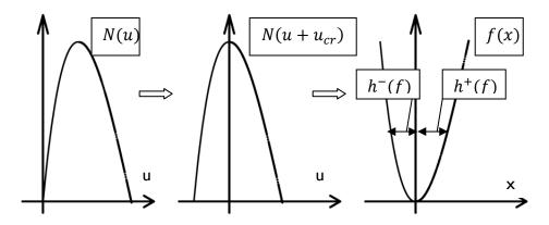
Fig. 3.11: Shifting and mirroring the force-displacement diagram
