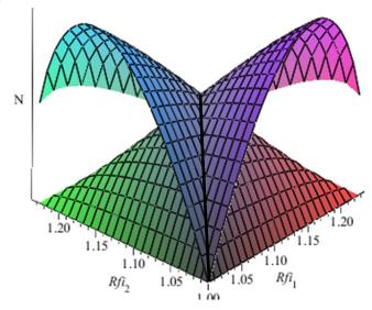
**Fig. 3.22:** Equilibrium path in function of the half-lengths of the elastic horizontal bars in the case of k=3, initial half-length:  $r_0=1$
