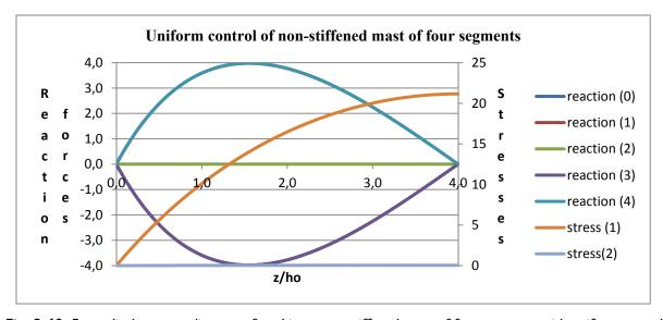
**Fig. 3.48:** Force-displacement diagram of packing a non-stiffened mast of four segments with uniform control  $(EA=100,h_0=1,r_0=1)$
