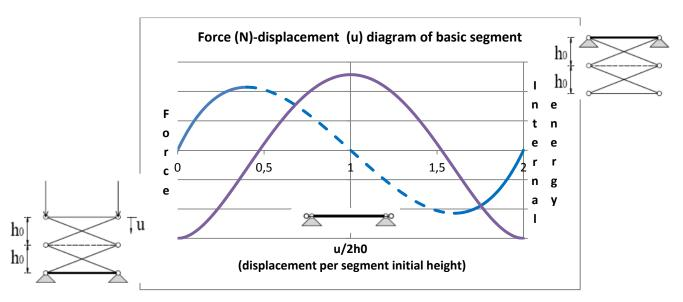
**Fig. 3.5:** Equilibrium path and internal energy during closure of boundary bars for basic segment with the 'post-packed phenomenon'
