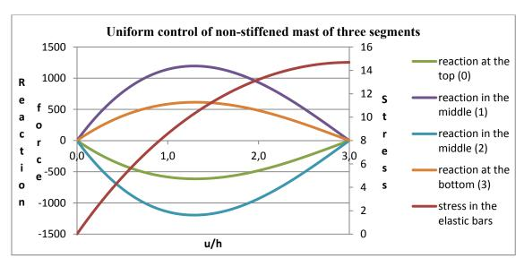
**Fig. 3.46:** Force-displacement diagram of packing a non-stiffened mast of three segments with uniform control  $(EA=100,h_0=1,r_0=1)$
