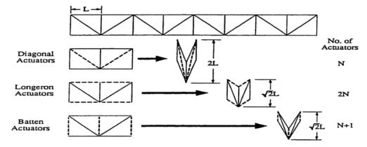
Fig. 2.40: Deployment of planar truss with length-variation [Mikulas et al., 1992]
