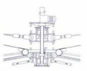
**Fig. 2.48:** Central spinder for prestressing the cables [Holgate, 1997]
