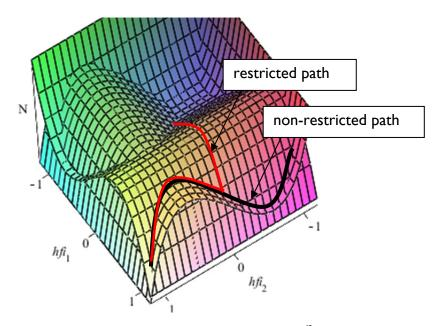
**Fig. 3.17:** Equilibrium paths in function of the half-heights of the segments  $(h_1^{\varphi}: half-height of top segment, h_2^{\varphi}: half-height of bottom segment) of planar deployable mast consisting of two segments taking into account the weight of the structure$
