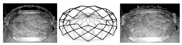
**Fig 2.29:** 3D model of retractable dome by multi-angulated elements and its physical model at the former Deployable Structures Laboratory [Kovács, 2004/2]
