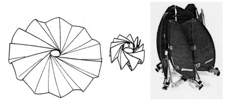
**Fig. 2.12:** Solid Surface Deployable Antenna and its wrapping fold pattern by the former Deployable Structures Laboratory by Guest and Pellegrino [DSL]
