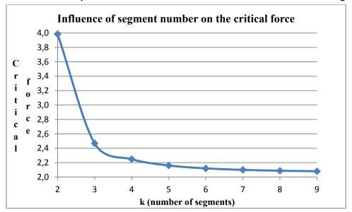
**Fig. 3.59:** Influence of segment number on the critical force of 'non-stiffened' masts for two different ratios of segment height and half-length of elastic bars (with logarithmic constitutive model, by FEAP)  $(EA = 100; h_0 = 1; r_0 = 1)$
