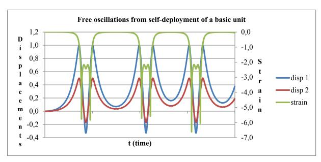
**Fig. 4.53:** Dynamic deployment of the basic unit of pentagonal antiprismatic mast: deployment sequence with (poorly captured) restriction of segment intersection initial self-stress ( $\sigma_{pre\_min} = 5000$ ) was smaller than  $\sigma_{pre\_min} = 5989$  ( $EA = 10\ 000$ ; R = 0.5; h = 0.5)
