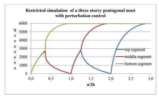
**Fig. 4.32:** Perturbation controlled restricted simulation of packing a three-storey pentagonal mast — stresses in the elastic bars during packing  $(EA_1=10\ 000;EA_2=9\ 990;EA_3=9\ 980;R=0.5;h=0.5)$
