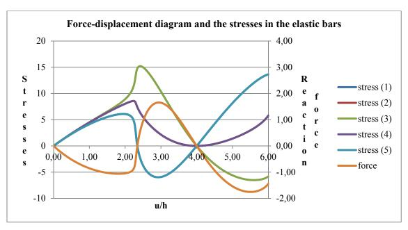
**Fig. 3.55:** Non-restricted packing simulation of non-stiffened mast of six segments by controlling only the displacements of the top nodes  $(EA = 100, h_0 = 1, r_0 = 1)$
