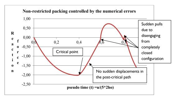
**Fig. 3.37:** Force-displacement diagram of five-storey planar pop-up mast controlled by numerical errors without the restriction of 'post-packed phenomenon' (packing sequence in Fig. 3.36, EA = 100,  $h_0 = 1$ ,  $r_0 = 1$ , downward force is negative)
