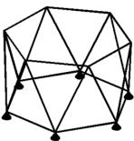
Fig. A1: Antiprismatic truss structure
