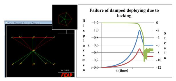
**Fig. 4.54:** Failure of damped deploying due to locking strain in the elastic bar (in green), nodal vertical displacements of the top facet (in blue) and of the middle polygon (in red)
