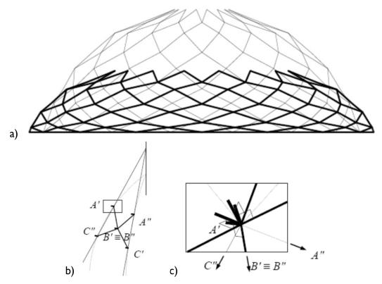
**Fig. 2.27:** a) Schematic model of Hoberman's Iris dome during deployment; b) angulated element on the tangent plane of a conical surface and c) four non-identical hinge axis at the connection of angulated elements [Kovács, 2004/2]
