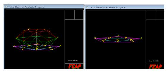
Fig. 4.33: Packing sequence of a three-storey 'alternately stiffened' mast with restricted simulation
