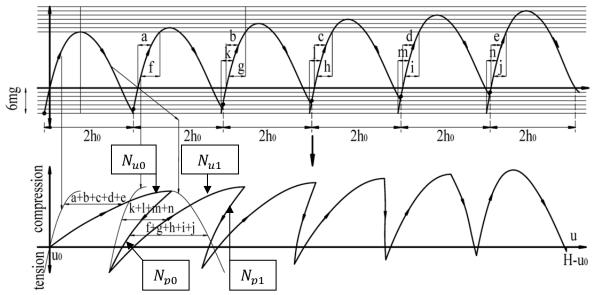
**Fig. 3.19:** Constructing the force-displacement diagram — restricted packing of planar deployable mast of six segments with self-weight
