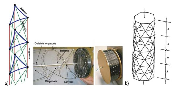
**Fig. 2.39:** Deployable masts: a) coilable mast by Mauch (Jet Propulsion Laboratory [JPL]) b) foldable mast by Hegedűs [1993]
