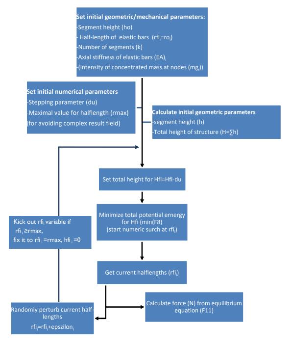
Fig. D1: methodology for tracing force-displacement diagram of multi-storey, 'alternately stiffened' masts
