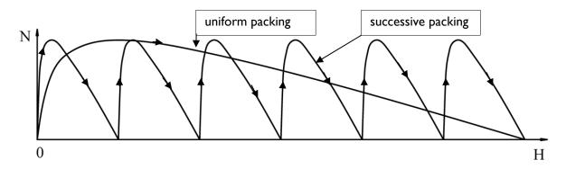
**Fig. 4.16:** Force-displacement diagram in the case of successive and uniform packing— restricted packing of antiprismatic deployable mast of six segments (notation: H: total height, u: displacement of the top nodes, N: packing force)
