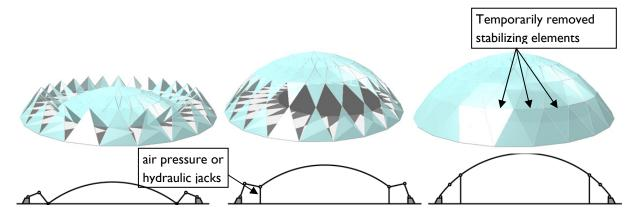
**Fig. 2.33:** Schema of the of the pantadome erection [Friedman et al., 2011/4] (in accordance with [Kawaguchi, 2002])
