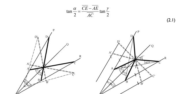
**Fig. 2.25:** a) Classic SLE and b) the simple angulated element (illustrated in accordance with [You and Pellegrino 1997])
