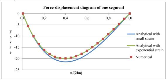
**Fig. 3.31:** Verifying numerical results with analytical solution – packing of basic segment (numerical results with logarithmic strain, analytical results with small strain formulation and with logarithmic strain  $EA = 500, h_0 = 1, r_0 = 1$ )
