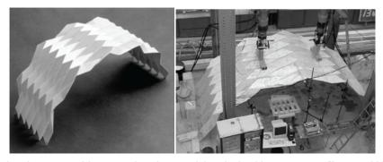
Fig. 2.13: Cylindrical paper and laminated timber model with the Miura pattern [Buri and Weinand, 2008]
