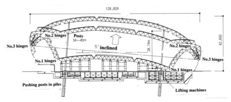
Fig. 2.35: Erection of Namihaya Dome [Kawaguchi, 2002]
