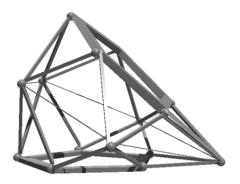
Fig. 4.3: Asymmetric freedom of motion of antiprismatic structures
