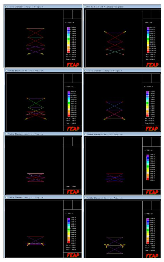
**Fig. 3.53:** Packing sequence from simulation of non-stiffened mast of four segments by successive control of double segments  $(EA=100,h_0=1,r_0=1)$
