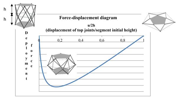
Fig. 4.7: Equilibrium path of basic deployable unit
