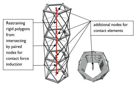
Fig. 4.30: Modeling restriction of 'post-packed phenomenon'
