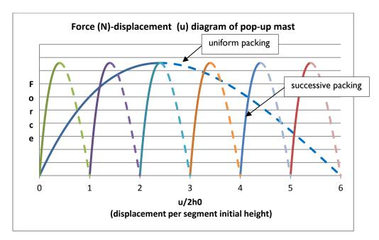
Fig. 3.6: 'Ideal' (uniform) and successive packing of planar deployable mast of six segments
