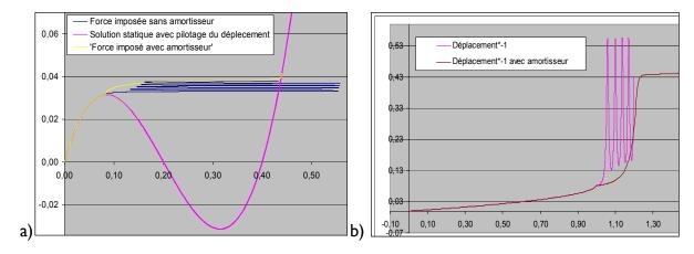
**Fig. B2** Force-displacement diagram with displacement control (in pink), with incremental force control (in yellow) and with additional damping (in blue) (a); Displacements in function of the time with (in brown) and without damping (in pink) with force control
