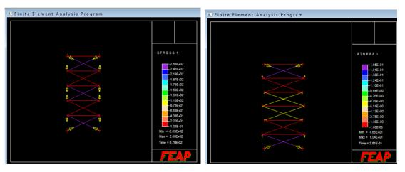
**Fig. 3.49:** Packing simulation of a non-stiffened mast of five and six segments with uniform control ( $EA = 100, h_0 = 1, r_0 = 1$ ), maximal reaction force at the top in case of five segments is  $R_{max}^{n5} = 361$  and the one of six segments is  $R_{max}^{n5} = 5,95$
