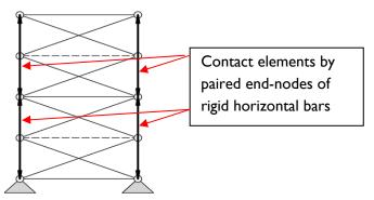
Fig. 3.38: Restricting 'post-packed phenomenon' with contact forces
