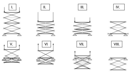
**Fig. 3.14:** Packing sequence of deployable mast of two segments without preventing 'post-packed phenomenon'
