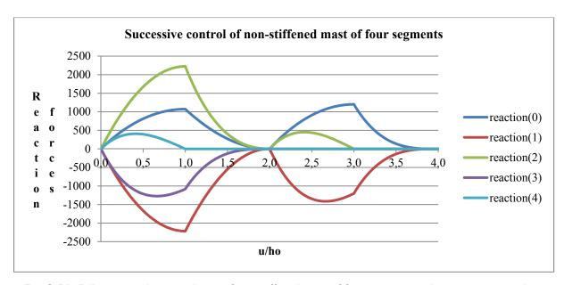
**Fig. 3.51:** Fallacious packing simulation of non-stiffened mast of four segments with successive control—reaction forces  $(EA = 100, h_0 = 1, r_0 = 1)$
