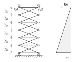
Fig. 3.43: Modeling the packing of non-stiffened mast by controlling only the displacement of the top nodes
