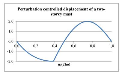
**Fig. 3.34:** Typical packing simulation of a two-storey planar mast without the restriction of 'post-packed phenomenon' controlled by the imperfection of axial stiffness values, downwards forces are negative  $(EA_1 = 100, EA_2 = 99.8, h_0 = 1, r_0 = 1)$
