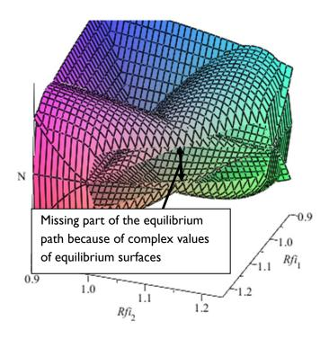
**Fig. 3.50:** Impossible closure of masts with odd number of segments — equilibrium path in function of the half-lengths of the elastic horizontal bars in case of k = 3 with the 'post-packed phenomenon'
