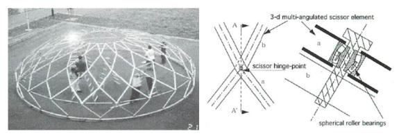
**Fig. 2.30:** Retractable dome opening on the spherical surface with telescopic ring, plan view and section of its scissor hinge [Kokawa, 2000]
