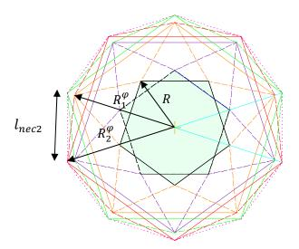
**Fig. 4.44:** Possible packing pattern of masts consisting of five segments or more (only in the case of odd number of segments)
