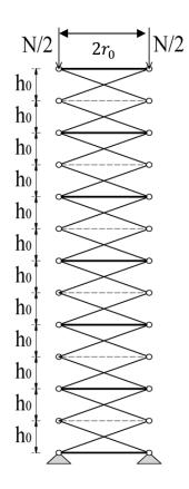
Fig. 3.1: Simplified planar deployable structure
