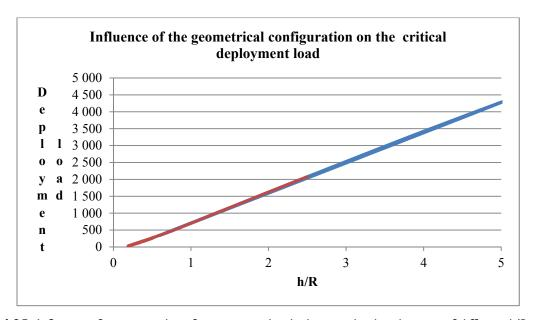
**Fig. 4.25:** Influence of geometrical configuration on the deployment load in the case of different h/R ratios (EA = 500; R = 0.5 (red)R = 1(blue)
