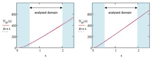
**Fig. 4.12:** Approximation for the critical force: critical force  $(N_{cr})$  in function of initial height/initial radius ratio (x = h/R), for pentagonal (on the left) and for 9-gonal segment (on the right) — exact solution with continuous line, linear approximation with dotted line (EA=100)
