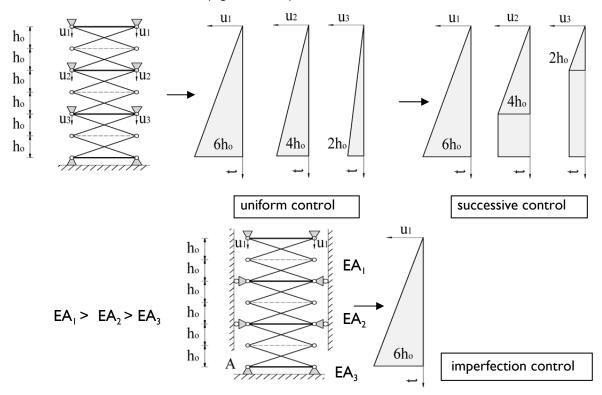
**Fig. 3.32:** Numerical models with different packing controls (uniform control, successive control, imperfection control, the non-uniform controls pack the segments successively from the bottom to the top)  $-u_i$  is the proportional vertical displacement of the i<sup>th</sup> boundary in function of the pseudo time (t)
