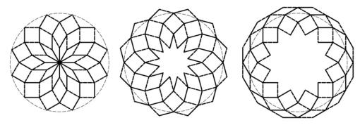
Fig. 2.28: Deployable sequence of a ring structure developed by Z. You and S. Pellegrino
