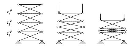
**Fig. 3.25:** Packing sequence without intermediate stiffening for k=4
