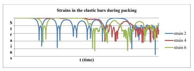
Fig. 4.50: Dynamic deployment of antiprismatic mast: strain in the elastic bars during deployment
