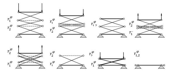
Fig. 3.28: Complete packing sequence of three-storey mast without restricting 'post-packed phenomenon'
