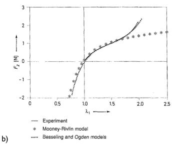
**Fig. E2:** Force-stretch diagram of rubber-like material from different constitutive models and from experiments [van den Bogert and de Borst, 1994]
