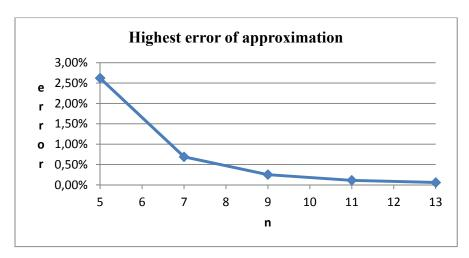
**Fig. 4.5**: Highest (at h/R = 0.5) error of the linear approximation for final stretching of elastic bars ( $\hat{\lambda}_{max}$ ) for different odd sided n-gons
