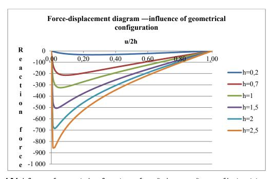
**Fig. 4.24:** Influence of geometrical configuration — force displacement diagram of basic unit in case of different h/R ratios (EA = 500; R = 0.5)
