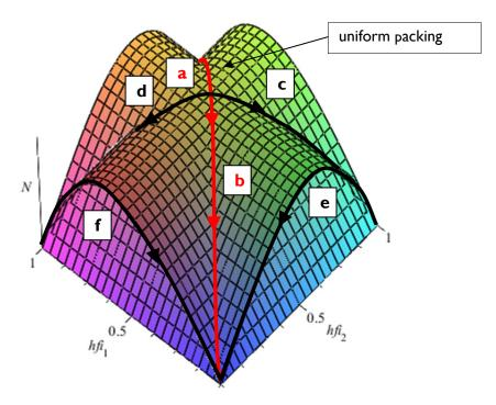
**Fig. 3.7:** Restricted equilibrium paths in function of the actual height of the segments  $(h^{\varphi})$  of planar deployable mast consisting two segments
