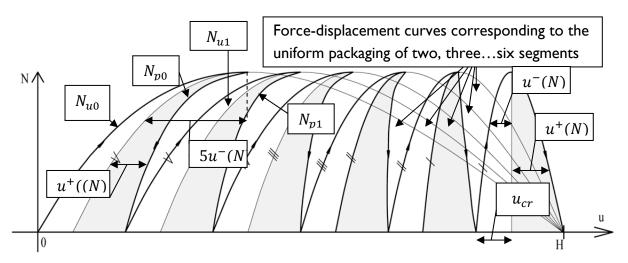
**Fig. 3.9:** Typical force-displacement diagram — restricted packing of planar deployable mast of six segments (notations: H: total height, u: displacement of the top nodes, N: packing force)
