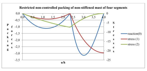
**Fig. 3.57:** Restricted packing of non-stiffened mast —force-displacement diagram and stresses during packing  $(EA = 100, h_0 = 1, r_0 = 1)$
