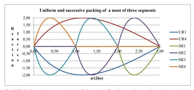
**Fig. 3.33:** Uniform and successive packing of 'alternately stiffened' mast —Reaction forces at the end nodes of the rigid horizontal bars (SRI-SR4: reaction forces from successive control respectively from the top to the bottom, URI, UR4: reaction forces from the uniform control at the top and at the bottom nodes, downward forces are negative  $(EA = 100, h_0 = 1, r_0 = 1)^2$
