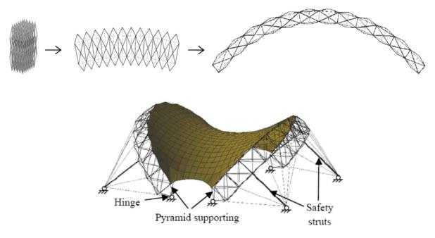
**Fig. 2.43:** Deployable arches by cable-strut-pantograph elements for a two-wing butterfly membrane structure: deployment of arches and the model of the structure [Tran et al., 2006]
