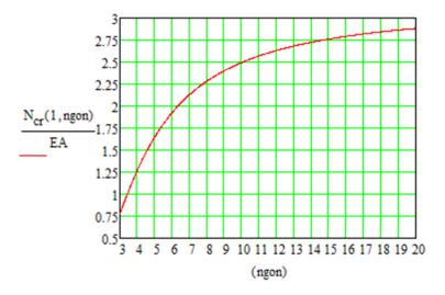
**Fig. 4.14:** Critical force  $(N_{cr})$  in function of the number of vertex of the polygon for h/R=1
