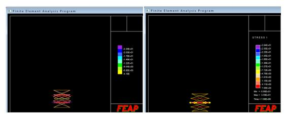
**Fig. 3.36:** Packing sequence controlled by the numerical errors of planar pop-up mast consisting of five segments, with simulation without the restriction of 'post-packed phenomena'  $(EA = 100, h_0 = 1, r_0 = 1)$
