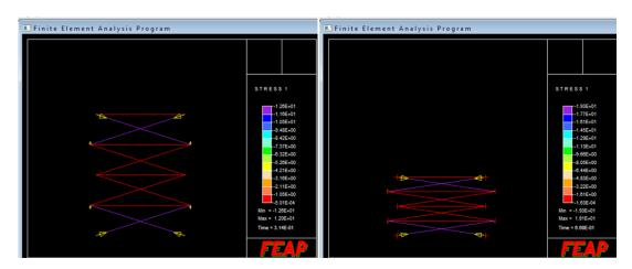
**Fig. 3.47:** Packing sequence of a non-stiffened mast of four segments with uniform control ( $EA = 100, h_0 = 1, r_0 = 1$ )
