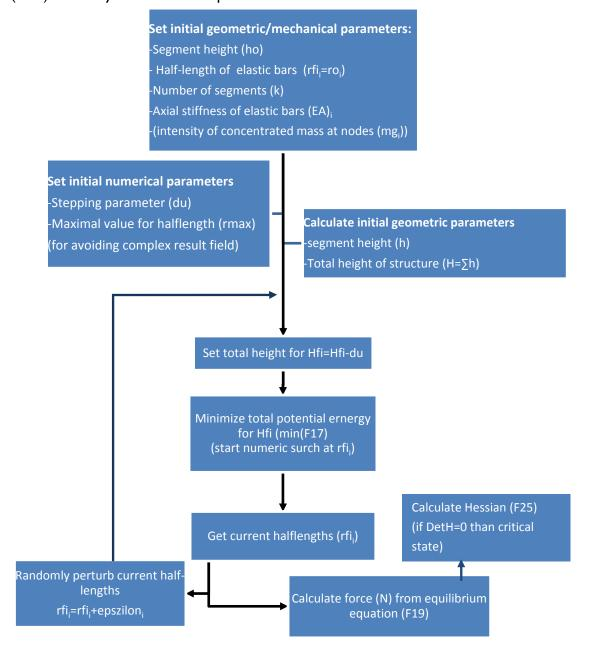
**Fig. D2:** Methodology for tracing force-displacement diagram of multi-storey, 'non-stiffened' masts until the first segment closure
