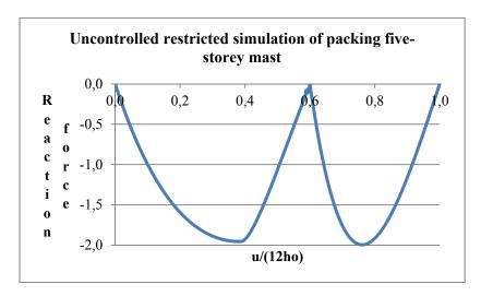
**Fig. 3.42:** Force-displacement diagram of five-storey planar pop-up mast controlled by numerical errors (packing sequence in Fig. 3.41, EA = 100,  $h_0 = 1$ ,  $r_0 = 1$ , downward force is negative)
