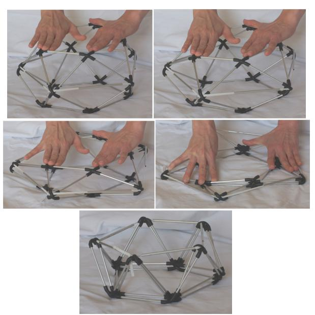
Fig. 5.2: Difficult control of non-stiffened pentagonal unit
