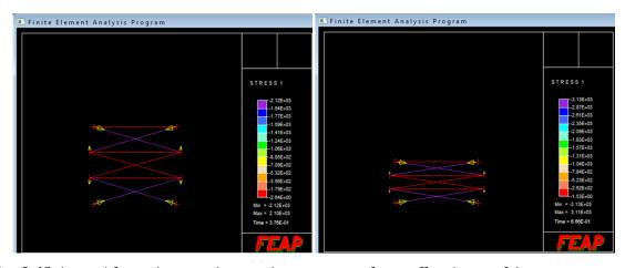
**Fig. 3.45:** Internal forces during packing: packing sequence of non-stiffened mast of three segments with uniform control  $(EA = 100, h_0 = 1, r_0 = 1)$
