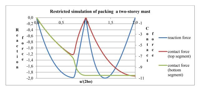
**Fig. 3.39:** Force-displacement diagram of packing a two-storey mast: restricted simulation with contact forces between the end nodes of rigid horizontal bars and packing control by imperfection of axial stiffness values  $(EA_1 = 100, EA_2 = 99, h_0 = 1, r_0 = 1)$
