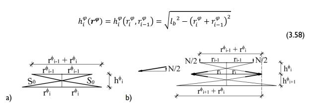
Fig. 3.21: a) Height of the non-stiffened mast from current bar-lengths and b) equilibrium of forces
