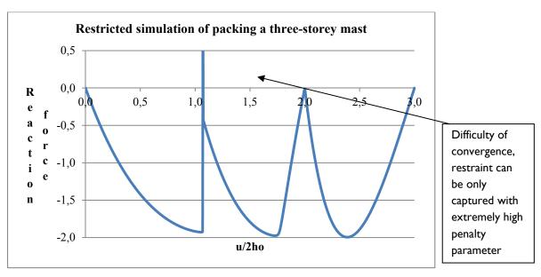
**Fig. 3.40:** Force-displacement diagram and the associated contact forces between the end nodes of rigid horizontal bars of packing two-storey mast with restricted simulation controlled by imperfection of axial stiffness, ( $EA_1 = 100, EA_2 = 99, EA_3 = 98 \ h = 1, r_0 = 1$ )
