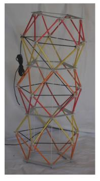
Fig. 5.7: Deployment control by one single cable (black stream: active cable, white strings: passive cables)
