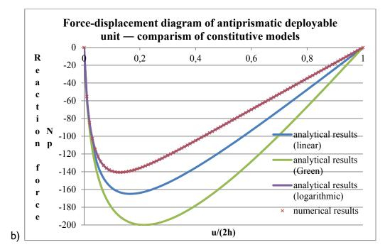
**Fig. 4.20:** Comparison of different constitutive models: stresses/E in function of the stretches analytical and numerical results (pentagonal unit, EA = 500; h = 0.5; R = 0.5)
