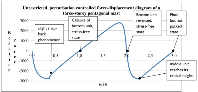
**Fig. 4.28:** Force-displacement diagram of a three-storey pentagonal mast — perturbation-controlled unrestricted simulation
