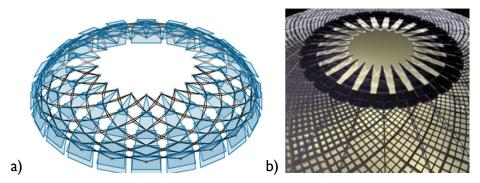
**Fig. 2.31:** Cover of retractable structures with sliding panels by Hoberman: a) schematic model for covering the iris dome (Happold and Hoberman) and b) model of the dome of Abu Dhabi's international airport, United Arab Emirates, 2006 (Kohn Pedersen Fox Architects) [Hoberman]
