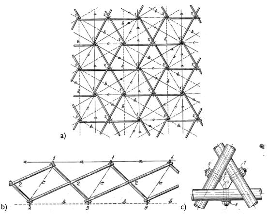
**Fig. 2.19:** Details of Pinero's reticular 3D structure patent: a) plan view of opened structure; b) fragmentary view; c) connection of three rods of the structure to an intermediate coupling [Piñero, 1965]
