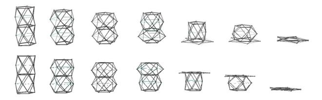
Fig. 4.19: Typical restricted packing sequences of antiprismatic deployable mast of two segments
