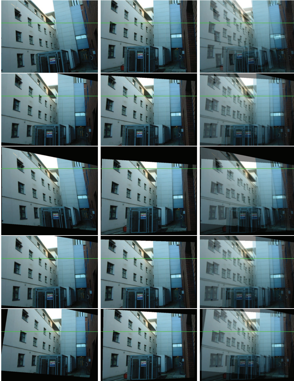
Figure 7.2: Image pair “Arch” rectified by different methods. From top to bottom: original images, proposed method, Hartley method, Fusiello et al. method and Mallon et al. method. A horizontal line is added to images to check the rectification. The third column represents an image average of each pair.
