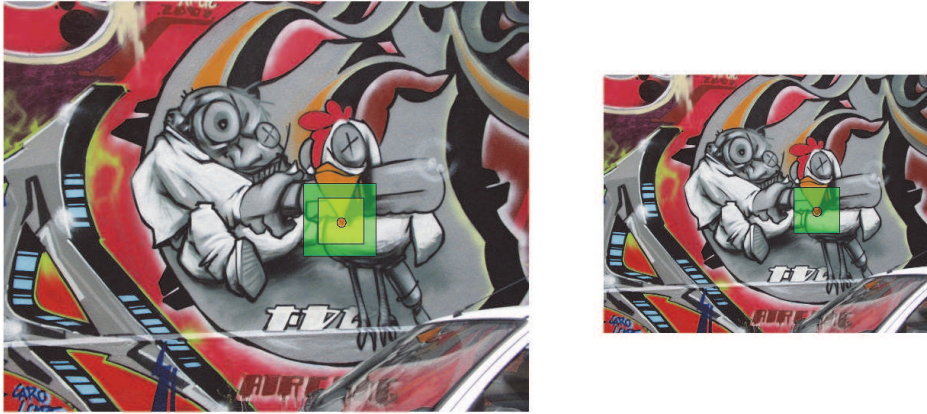
Figure 8.5: The right image is a 2^{2/3} -subsampling of the left image. A feature in the right image with blur \sigma corresponds to a feature with \sigma \times 2^{2/3} in the left image. The fixed-size descriptor gives evidently different patches for a common feature in both images (yellow patch in the left image via green patch in the right image). The two patches (in green) look almost the same by using a descriptor with size proportional to the blur.
