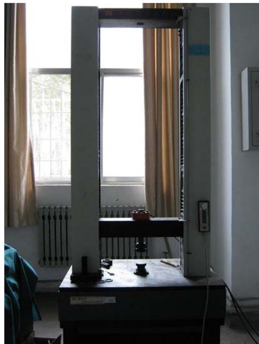
Figure 3.6 Universal tension-compression CSS88010 machine
