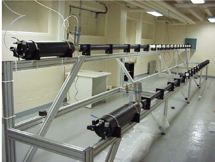
Figure 3.2. The Nylon Hopkinson bars with diameter  $\Phi=60\text{mm}$
