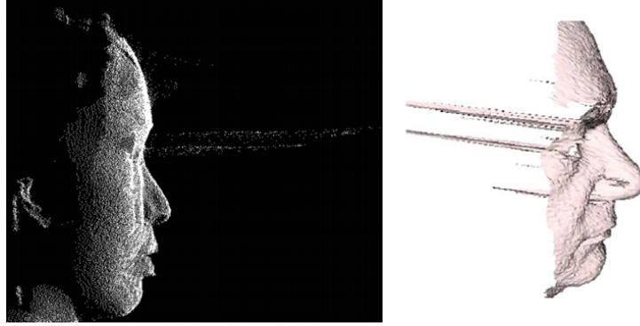
Figure 2.3: Example of spikes artefacts on 3D model acquired by laser based scanners. [Mian et al. 2007, Bowyer et al. 2006]
