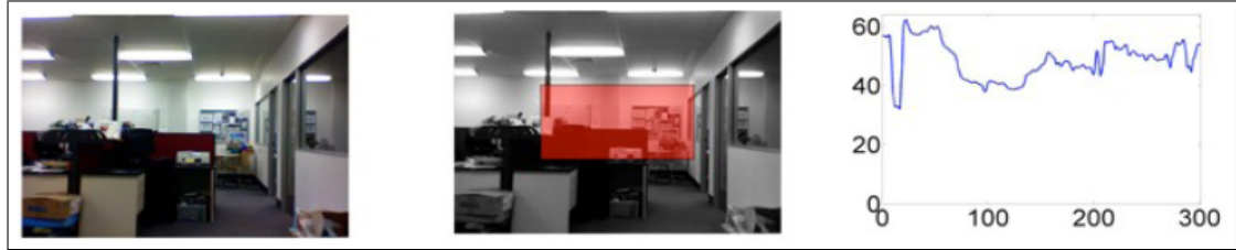
Figure 4.6: Acquired image (left), greyscale image and selected sub-window (middle), and the corresponding Image Array (right), from (55).
