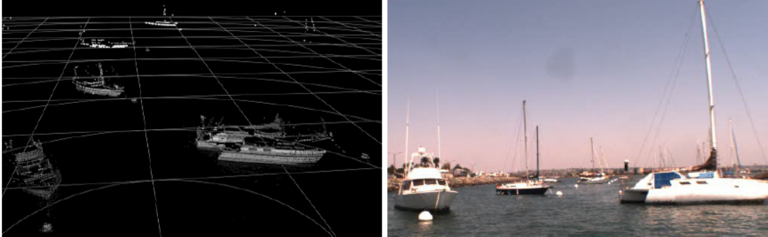
Figure 2.23: Maritime data acquisition using HDL-64E (from (28))
