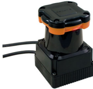
Figure 2.4: The Hokuyo UTM-30LX lidar
