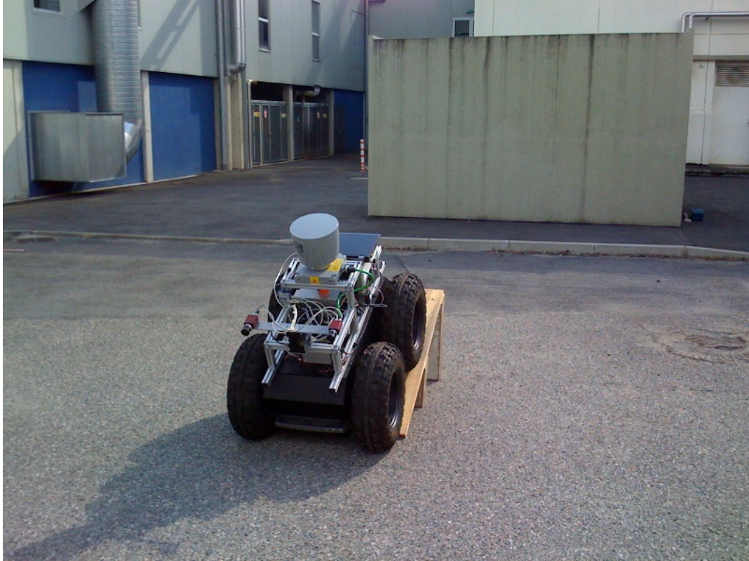
Figure 3.3: Robot Mana on the wooden ramp scanning the calibration target
