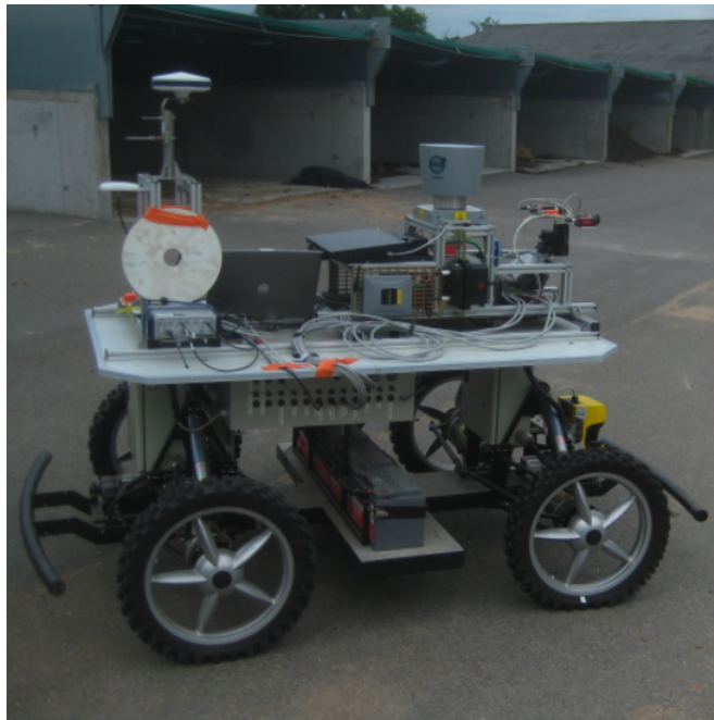
Figure 5.12: The robot Robufast equipped with the Velodyne lidar device and other sensors.
