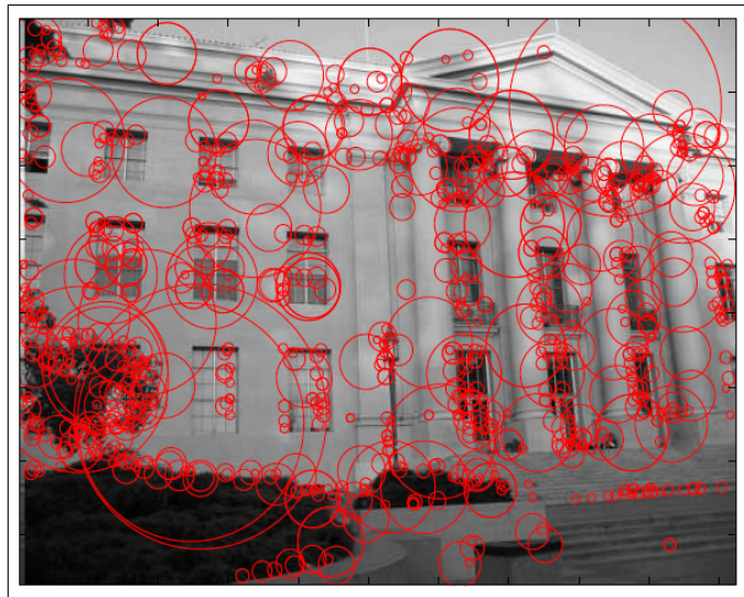
Figure 4.7: SIFT features: size of the circle is proportional to scale of the feature, from (96).
