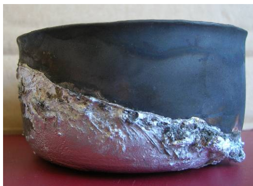
Figure III.32. Cups partially immersed from the bottom in the liquid zinc bath at 480°C during 2 minutes
