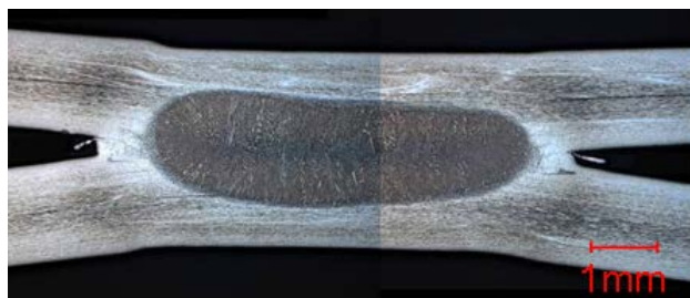
Figure V.7. Cross section observation of spot weld with 3mm gaps between sheets
