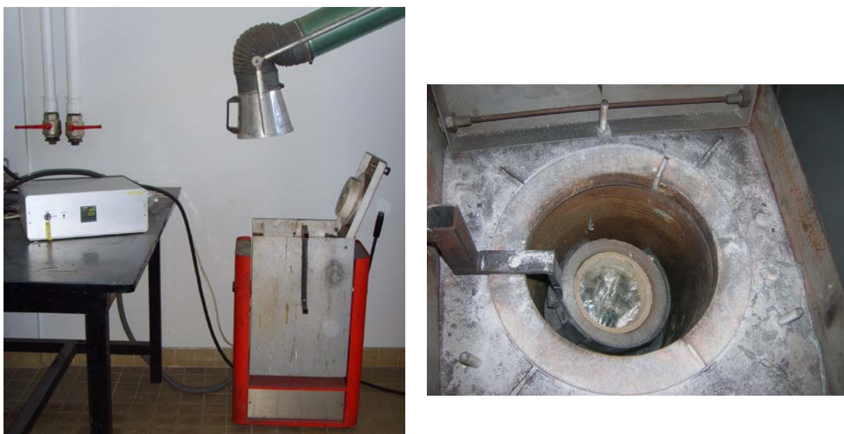
Figure II.6. Furnace used for galvanizing
