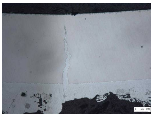
Figure III.38. Optical micrograph of section of cup immersed 7 minutes at 460°C
