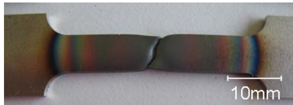
Figure III.9. Cold rolled specimen after tensile test at 600^\circ\text{C} , 1.3 \cdot 10^{-1} \text{ s}^{-1}
