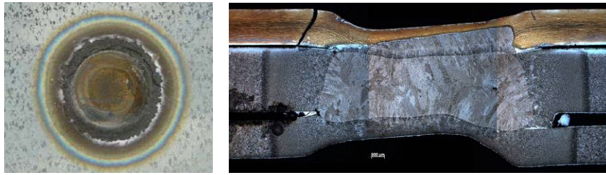
Figure 0.1. Cracks observed on dissimilar spot weld TWIP 1,2mm/Usibor 2,5mm/Usibor 1,75mm [BOU 07]
