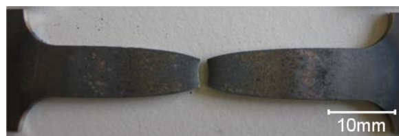
Figure III.4. Specimen after tensile test at 900°C, 1.3 \cdot 10^{-1} \text{ s}^{-1}
