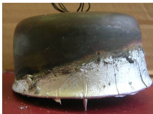
Figure III.34. Cups partially immersed from the rim in the liquid zinc bath at 480°C during 2 minutes
