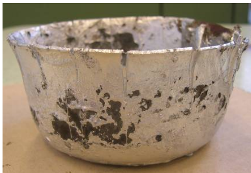
Figure III.31. Cup after immersion in the liquid zinc bath at 470°C during 7 minutes
