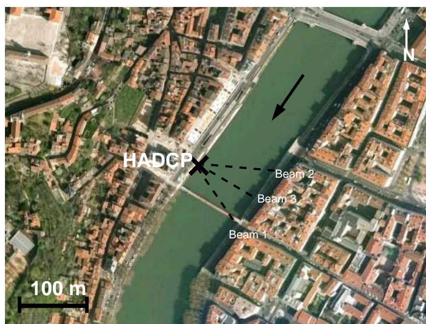
Figure 3.12: Aerial photograph of the Saint-Georges study site taken from Google Maps. The location of the side-looking ADCP is marked by an x and the direction of flow is indicated with an arrow.
