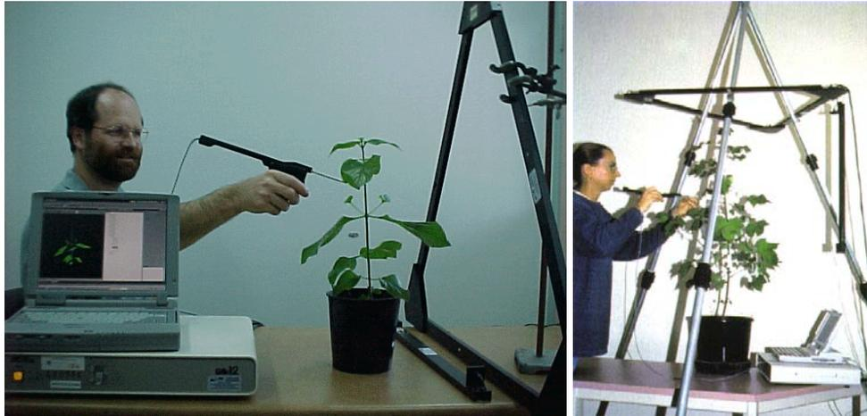
**Figure 5** Measurement of plant architecture using ultrasonic digitiser
