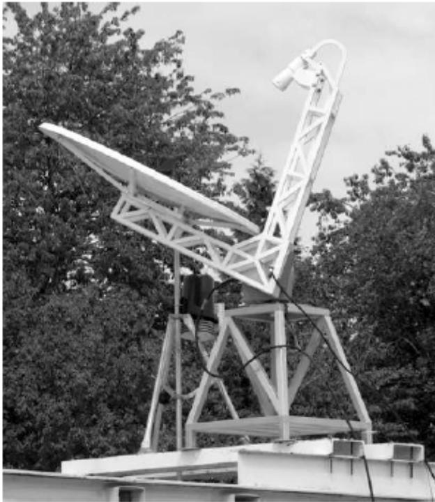
**Figure 1:** Picture of the CURIE offset antenna at the top a shelter at the SIRTa site (Ecole Polytechnique Palaiseau, France). The antenna is fixed to a positioning system at the left of the picture.
