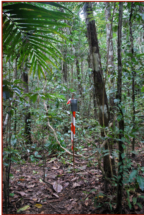
Figure 11.2 Shielded data-logger on the top of a 1-m high pole in forest interior.
