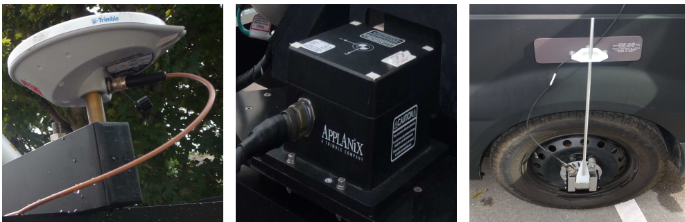
(a) Global Positioning System (GPS). (b) Inertial Measurement Unit (IMU). (c) Odometer.
