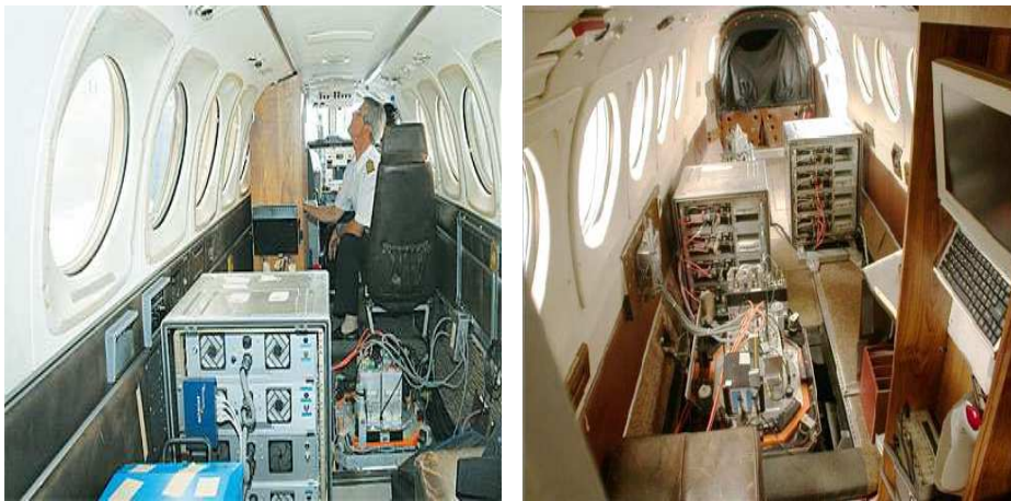
(b) Officer that controls aerial acquisition (c) Similar scene observed from the opposite system from an on-board station (back-site point of view. The central camera is ground) connected to the central camera installed in the floor hatch. (foreground).
