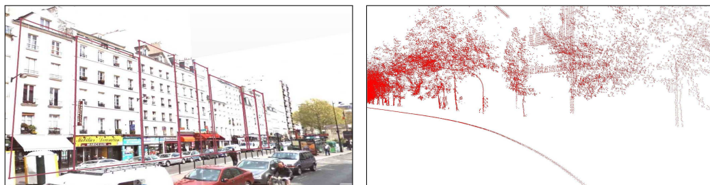
(d) Case 1: No presence of significant occlusions detected in front of the facade model. The facade image should be quasi-clean. A direct texturing can be achieved by using a segmented panoramic image. (e) Case 2: Presence of significant occlusions in front of the plane illustrated in Figure 5.14(a). The facade image should be occluded. A multi-view image mosaicking should be envisaged in order to generate occlusion-free facade textures.
