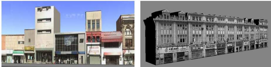
(c) Generated street facade models with quadrilateral facade representation (as LOD shown in Fig. 5.4(a)). (d) Generated street facade models with polygonal facade representation (as LOD shown in Fig. 5.4(b)).
