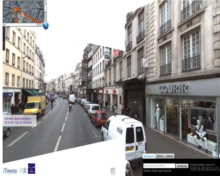
Figure 1.3: Google like Street-viewer developed to the IGN. Assembly of optical images that constitutes high resolution panoramic images useful for the street visualization and navigation at 360°.
