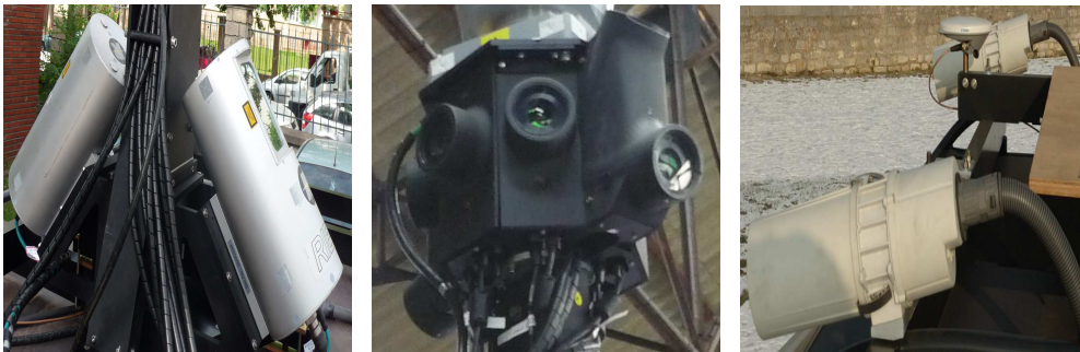
(a) 2D range laser sensor (two cylinders) sloped to the facade top directions. (b) Optical cameras organized at 360^\circ to cover the surrounding scene (omnidirectional device). (c) Optical cameras organized in stereoscopic pair.
