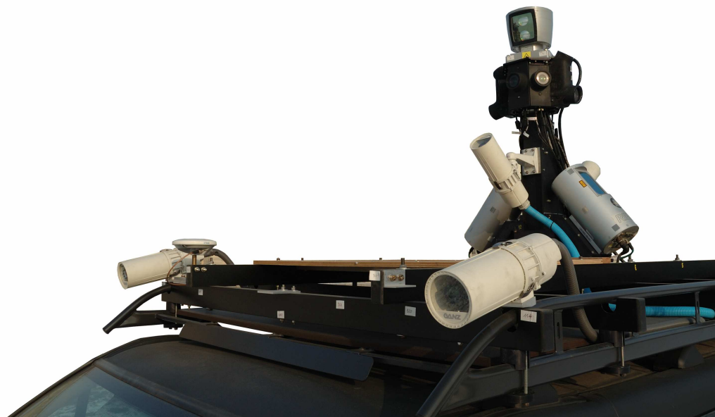
Figure 3.4: View of a set of devices located at the roof of the vehicle.
