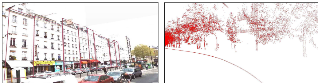
(d) Case 1: No presence of significant occlusions detected in front of the facade model. The facade image should be quasi-clean. A direct texturing can be achieved by using a segmented panoramic image. (e) Case 2: Presence of significant detected occlusions in front of the plane illustrated in Figure 5.14(a). The facade image should be occluded. A multi-view image mosaicking should be envisaged in order to generate occlusion-free facade textures.
