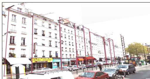
(d) Case 1: No presence of significant occlusions detected in front of the facade model. The facade image should be quasi-clean. A direct texturing can be achieved by using a segmented panoramic image. (e) Case 2: Presence of significant detected occlusions in front of the plane illustrated in Figure 5.14(a). The facade image should be occluded. A multi-view image mosaicking should be envisaged in order to generate occlusion-free facade textures.
