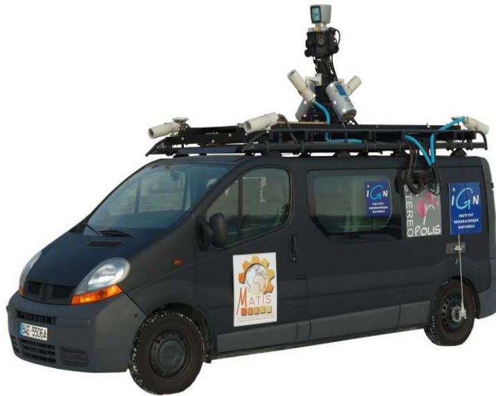
Figure 1.2: IGN street Mobile Mapping System.
