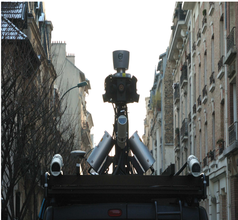
Figure 3.8: On-drive acquisition of street raw data by using the IGN Mobile Mapping System in dense urban environment (longitudinal view). Example of high disparity in facade size, alignment and visibility from one street side to the other. Typical sensor configuration employed in our case.
