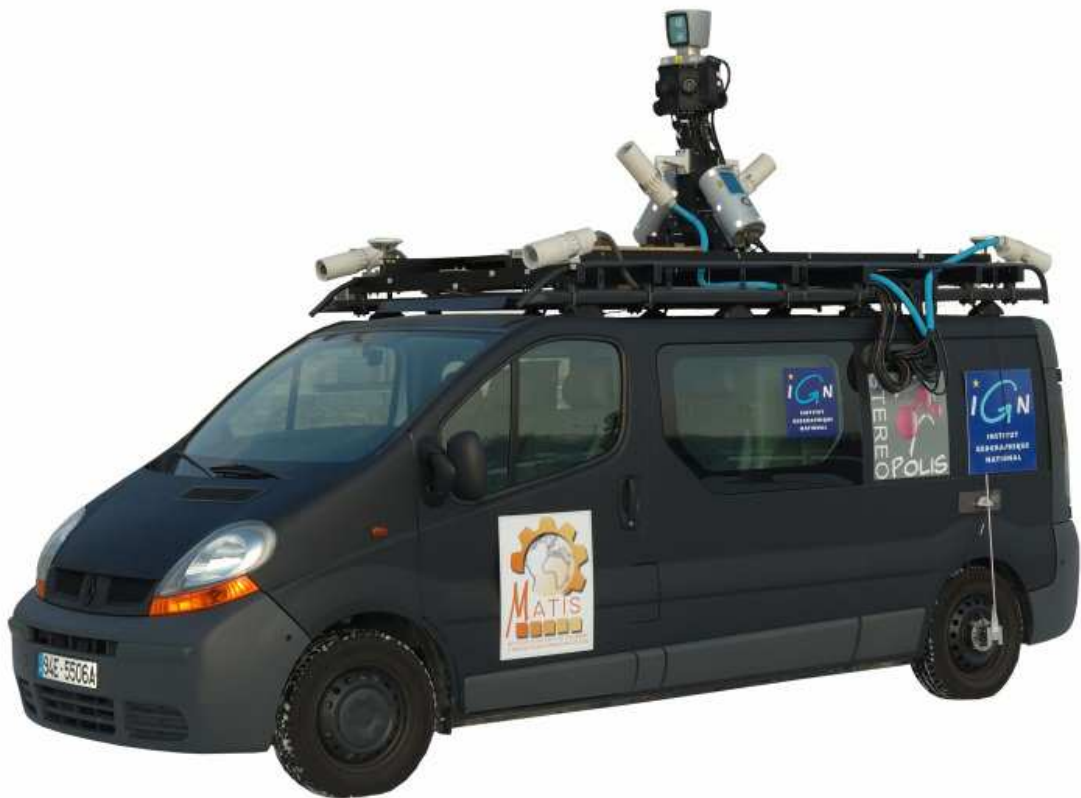
Figure 3.3: IGN Street Mobile Mapping System.
