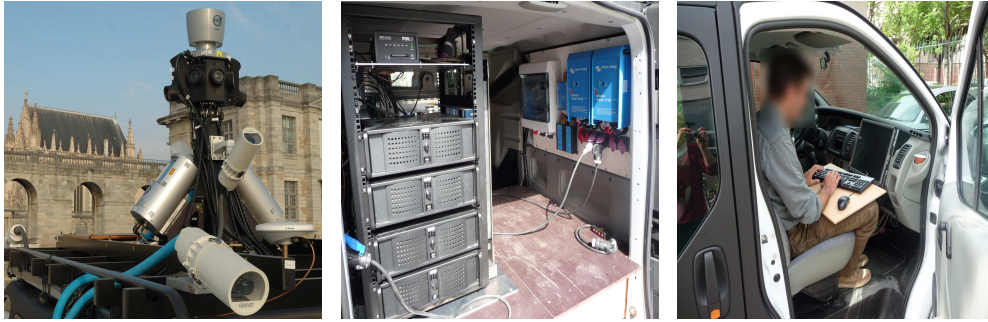
(a) To the roof, instruments of measurements have been mounted on a mast. (b) At the back, a unit of secure data storage and a power system have been fixed. (c) At the passenger side, a station control with an on-board computer has been installed.
