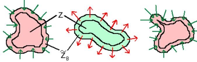
Figure 3: Principle of the reduction. Red area and arrows (resp. green area arrows) denote the flow which get in (resp. out of)  $Z_B$ . The nodes from  $Z$  are removed since  $Z$  satisfies (38). Remaining nodes are typically located in the narrow band  $Z_B \setminus Z$ .
