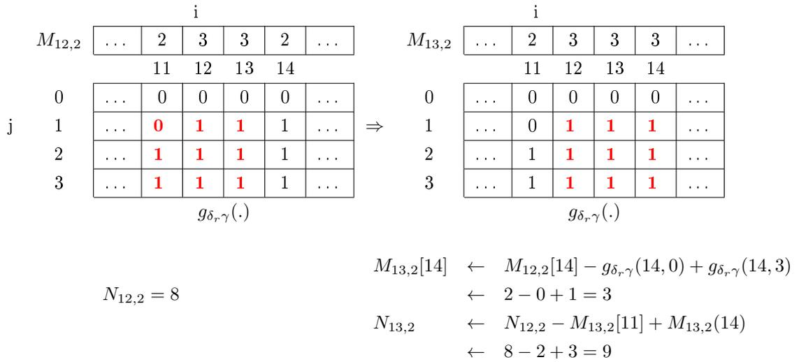
Figure 6: Illustration of the incremental algorithm for building  $\mathcal{G}$  on a 2D image with  $r = 1$ ,  $\gamma = 1$  and  $\eta = 1$ . In this example, only the node corresponding to the pixel  $p = (13, 2)$  is added to  $\mathcal{G}'$  since  $|N_{13,2}| = (2r + 1)^2 = 9$ .
