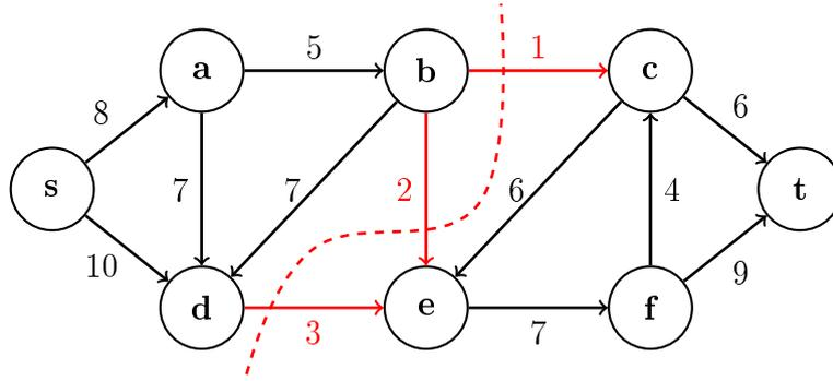
Figure 4: A minimum s-t cut  $\mathcal{C}^*$  of a weighted directed graph, whose weight is equal to 6. The minimum s-t cut  $\mathcal{C}^*$  consists of the set of edges  $\{(b, c), (b, e), (d, e)\}$ .
