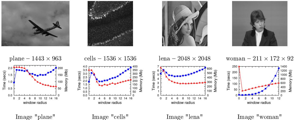
Figure 8: Influence of window radius (bottom row) for segmenting 2D and 2D+t images (top row) with a  $TV+L^2$  model in connectivity 1. On the bottom row, blue curve with squares and red curve with triangles correspond respectively to execution time and to the amount of memory allocated for the graph. Standard graph cuts correspond to  $r = 0$ .
