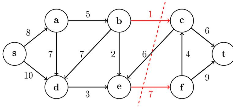
Figure 3: An s-t cut of a weighted directed graph whose weight is equal to 8. The red dashed line denotes the s-t cut  $\mathcal{C}$  splitting  $\mathcal{V}$  into two disjoint sets of nodes  $\mathcal{S} = \{s, a, b, d, e\}$  and  $\mathcal{T} = \{c, f, t\}$ . Thus,  $\mathcal{C}$  consists of the set of edges  $\{(b, c), (e, f)\}$ .
