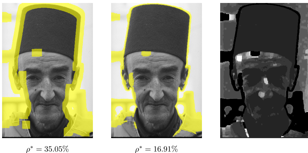
Figure 7: Illustration of memory gain brought by the adaptive algorithm (middle) versus the incremental algorithm (left) for segmenting a 2D image with a TV+L^2 model in connectivity 1. In this experiment we set r = 13 and r_{max} = 13 . On the left and middle images, the reduced graph is superimposed in yellow by transparency. In the right image, any pixel p is assigned with r_p^{min} . Brighter pixels are the nodes which can be removed with a larger window radius r and black pixels belong to \mathcal{G}' .
