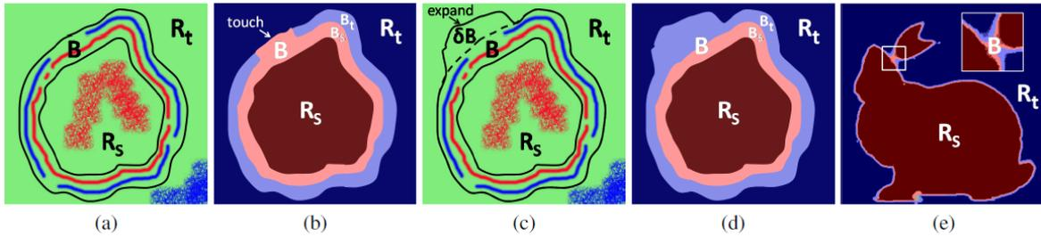
Figure 3: Touch-Expand algorithm maintains a band  $B$  and subgraphs  $R_s$  and  $R_t$  as in (a) where red (resp. blue) pixels/nodes are linked to terminal  $s$  (resp.  $t$ ). If a min-cut in the band  $B$  results in a touch as in (b), then  $B$  is expanded (c). If not as in (d), the min-cut is guaranteed to be the same than on the whole graph and the algorithm stops. (e) shows a band at convergence for a real problem. The picture is courtesy of [LB07].
