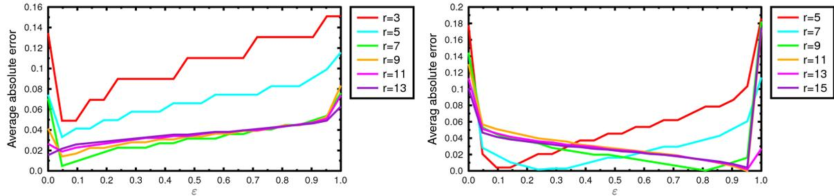
Figure 18: Evolution of the average absolute error between the empirical upper bound  $\eta_{max}^{emp}$  and the statistical upper bound  $\eta_{max}$  versus the parameter  $\varepsilon$ , for a fixed amount of noise  $\xi = 0.05$  (left) and  $\xi = 0.2$  (right). Color curves correspond to distinct window radii.
