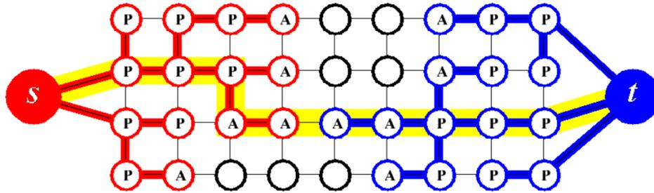
Figure 8: Representation of search trees  $A$  (red) and  $B$  (blue) at the end of the growing stage when an augmenting path (yellow line) is found. "A" and "B" labels resp. stand for active and passive nodes. Free nodes appear in black. The picture is courtesy of [BK04].
