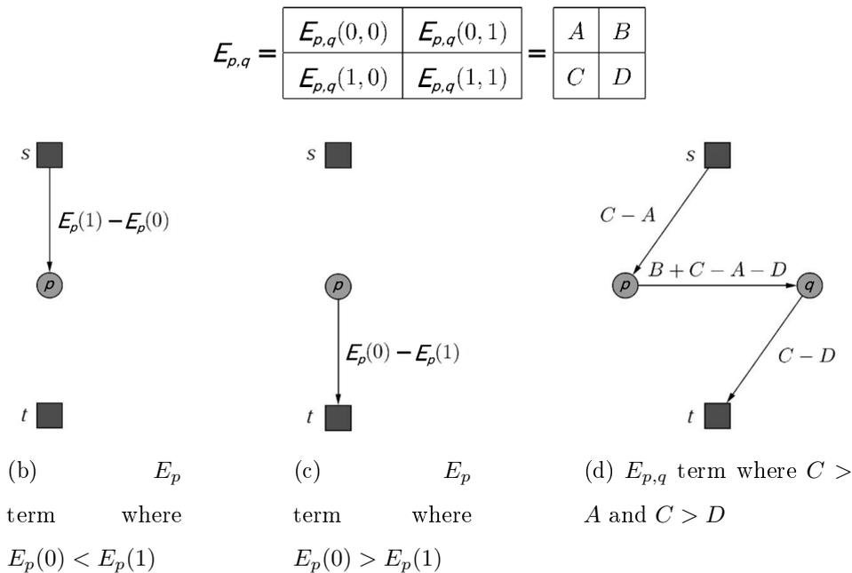
Figure 9: Graph construction in the binary case [KZ04].
