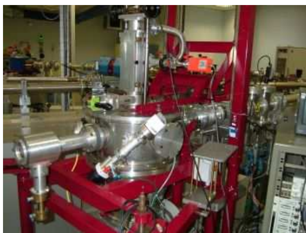
Fig. 42: AIFIRA facility: target chamber of the micrometric beamline.
