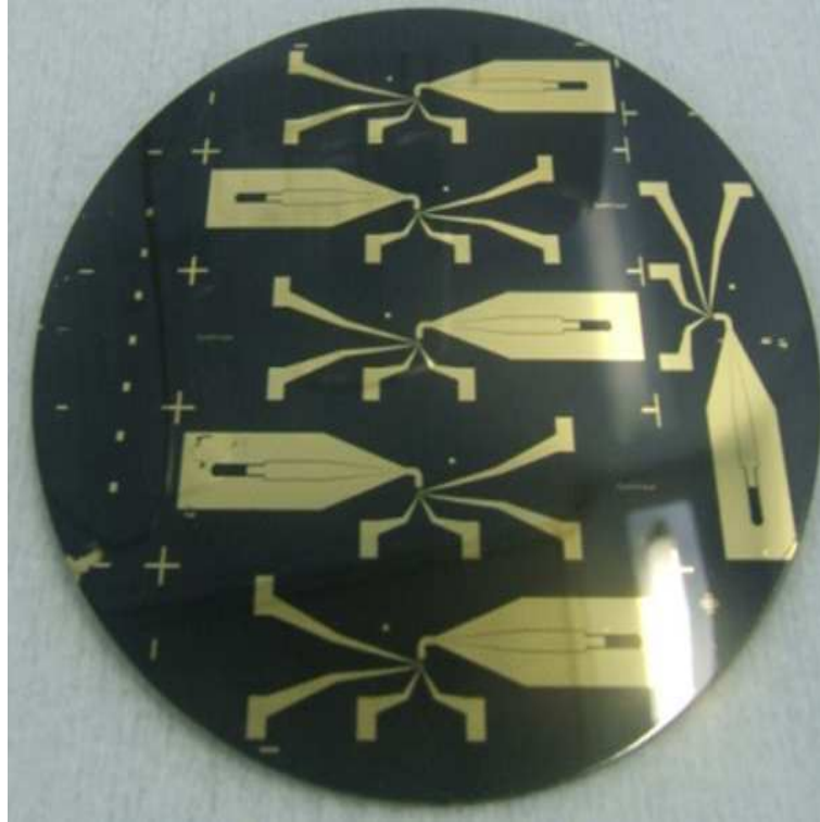
Figure 2.8: Optical photography of a 2 inch wafer after the fabrication of the antennas.
