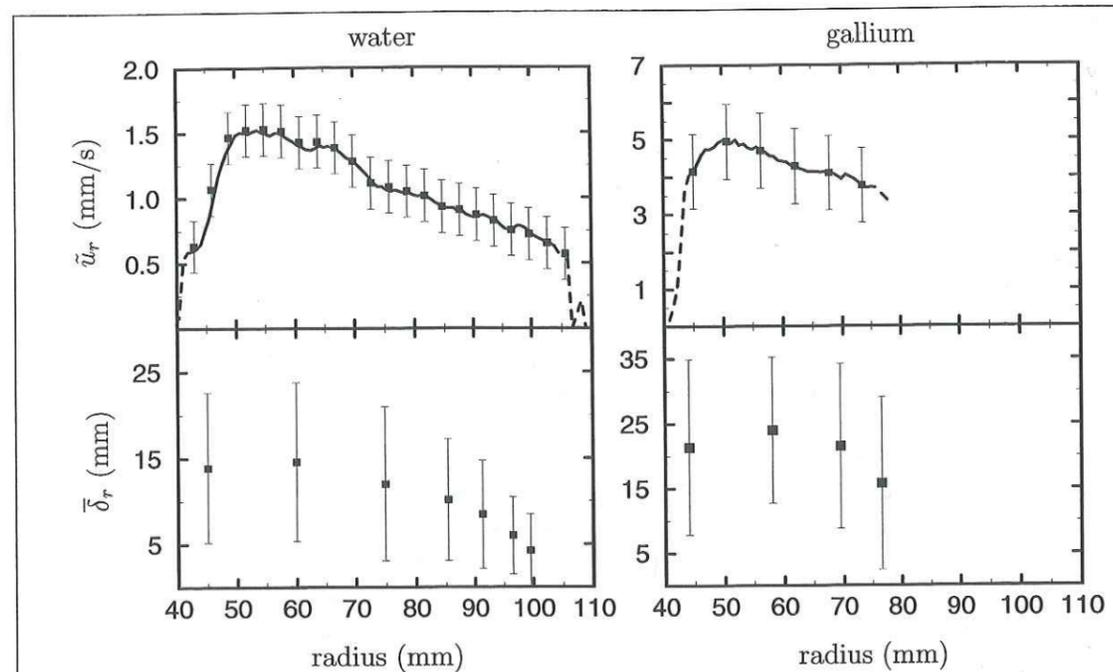
Figure 2.7: Mean properties for the flow extracted from patterns 3 and 4. Broken line in gallium plots of this figure and figure 2.8 highlights the region where the signal is saturated by multiple echoes due to the impedance contrast between copper and liquid gallium.
