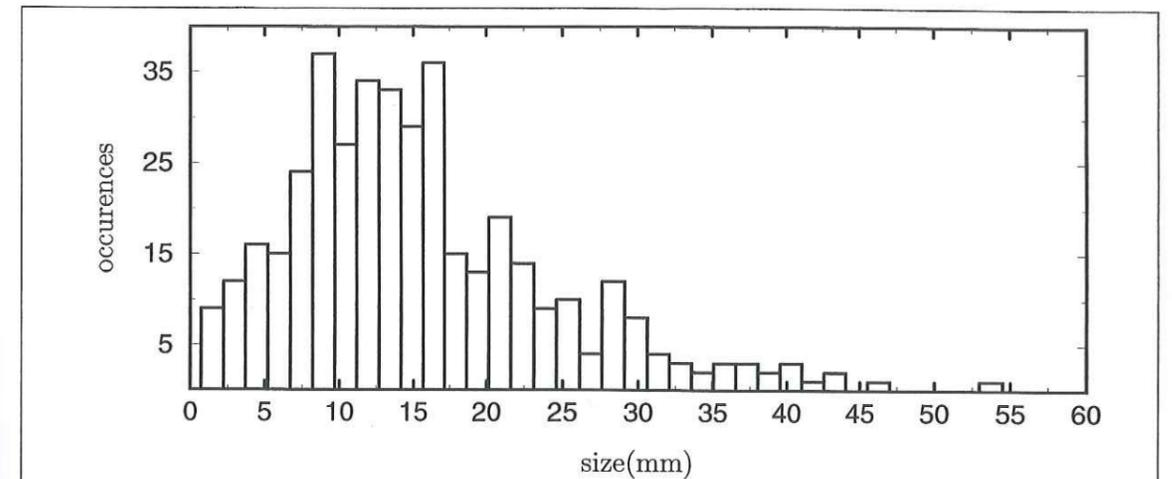
Figure 2.15: Histogram of the distribution of radial cell sizes in the convective flow, measured at radius 60 mm in water, for experiment of figure 2.5.3 (Ekman number is  $4.8 \cdot 10^{-6}$ , Rayleigh number is 26.6 times critical).
