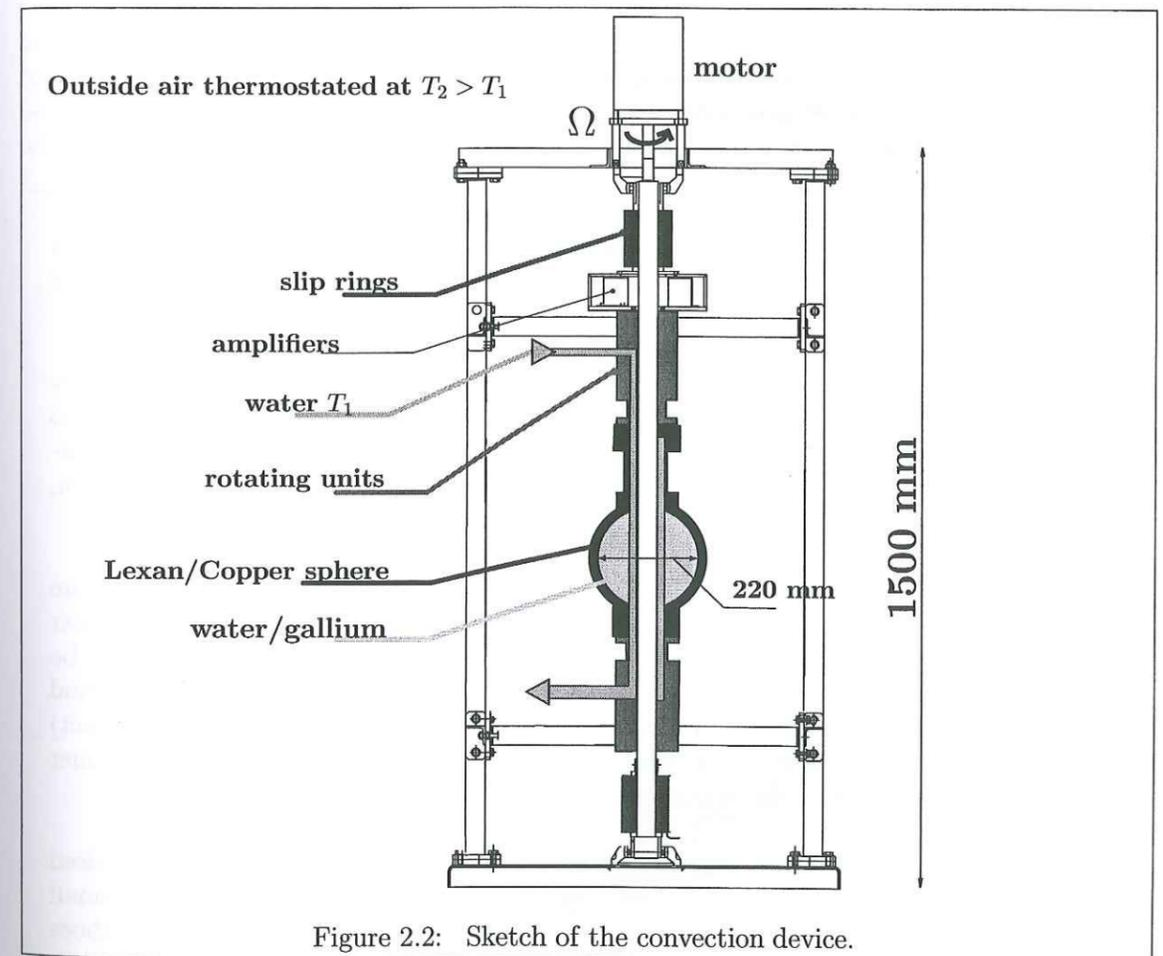
Figure 2.2: Sketch of the convection device.
