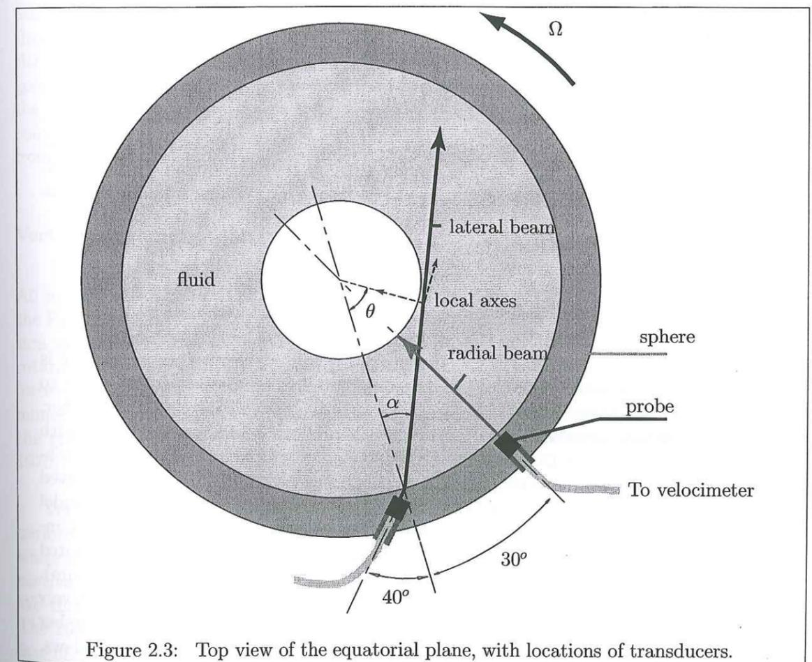
Figure 2.3: Top view of the equatorial plane, with locations of transducers.
