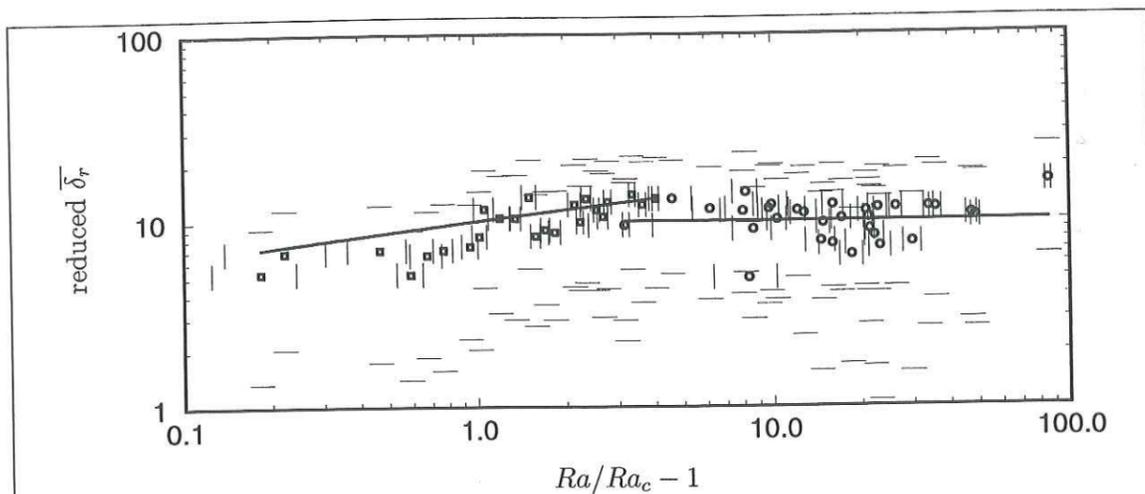
Figure 2.12: Reduced cell size for gallium (squares) and water (circles) experiments. The viscous scaling is tested for water experiments, the reduced cell size is therefore  $\bar{\delta}_r/E^{1/3}$ . The inertial scaling is tested for gallium experiments, the reduced cell size is therefore  $\bar{\delta}_r/(Ra_Q^{1/5} P^{-2/5} E^{3/5})$ . Black line in gallium corresponds to dependence  $y \sim (Ra/Ra_c - 1)^{1/5}$ . Black line in water is  $y \sim 1$ . Both prefactors are 10.
