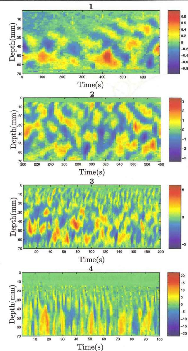
Figure 2.5: Time-depth radial velocity patterns. Velocities are expressed in millimeters per second. 1: performed in water, with  $Ra/Ra_c = 4.2$ ,  $E = 9.7 \cdot 10^{-6}$ ; 2: performed in water, with  $Ra/Ra_c = 22.2$ ,  $E = 9.7 \cdot 10^{-6}$ ; 3: performed in water, with  $Ra/Ra_c = 26.6$ ,  $E = 4.8 \cdot 10^{-6}$ ; 4: performed in liquid gallium, with  $Ra/Ra_c = 3.2$ ,  $E = 1.5 \cdot 10^{-6}$ .
