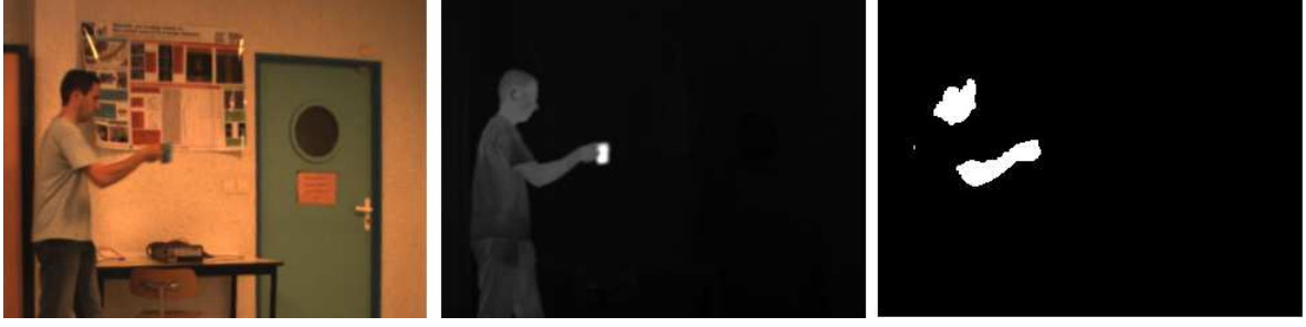
FIGURE 1.2 – left and center : color and temperature information of the scene - right : regions where g_1 = 1 in white
