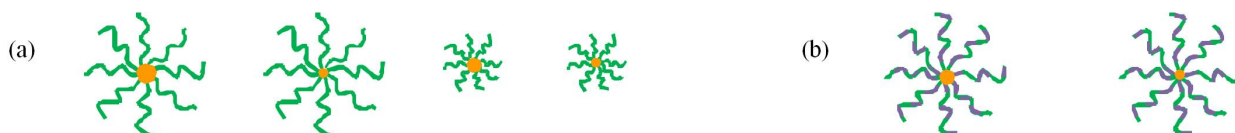
Figure 2.14: Thermoresponsive gold nanoparticles synthesized by "Grafting-to" via the one-step technique:(a)Au-PNIPAM ( M_w = 7861 - 29650 g.mol ^{-1} and D = 4.5 - 8.0 nm) and (b) Au-PNIPAM-co-NPAM (NIPAM:NPAM = 2.4:1 to 1:1 and D = 2.9 - 5.3 nm).
