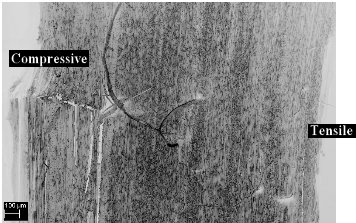
Figure 5.3 SEM micrograph of whole fracture surface of untreated T700/CNT fiber composite
