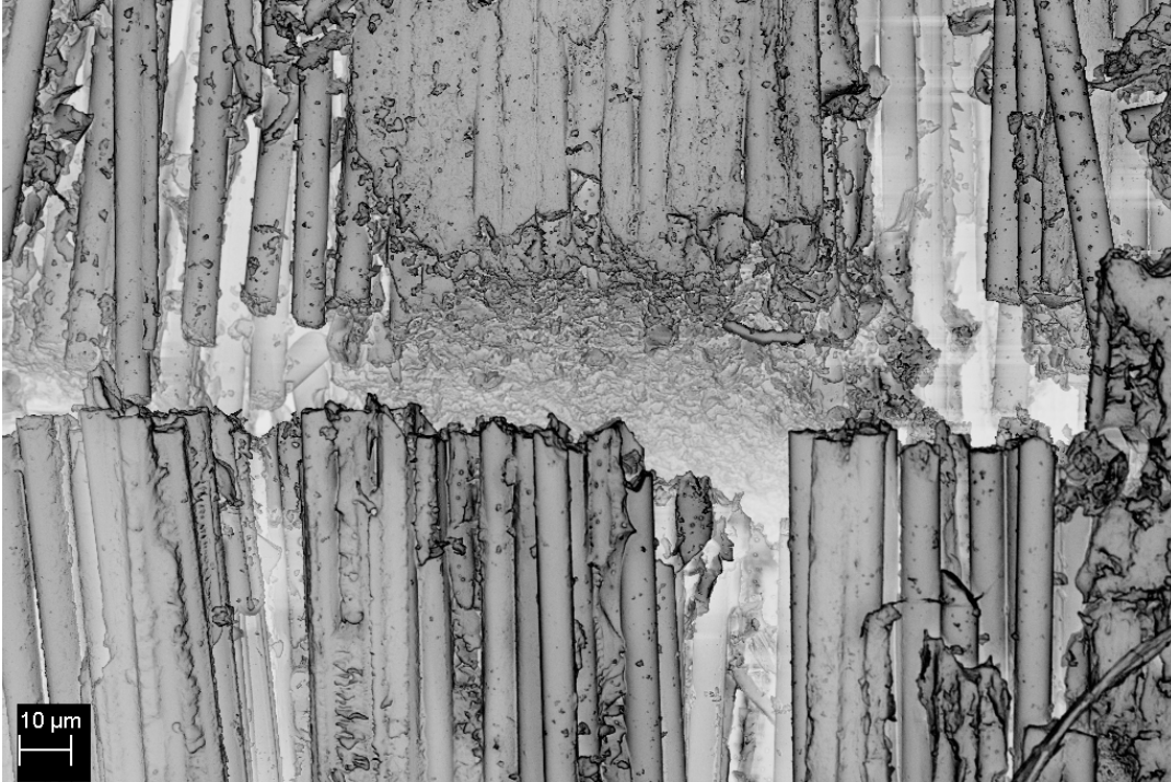
Figure 5.18 SEM micrograph of fiber matrix interface from compression area for pyrrole (1400 W) treated T700/CNT fiber composite
