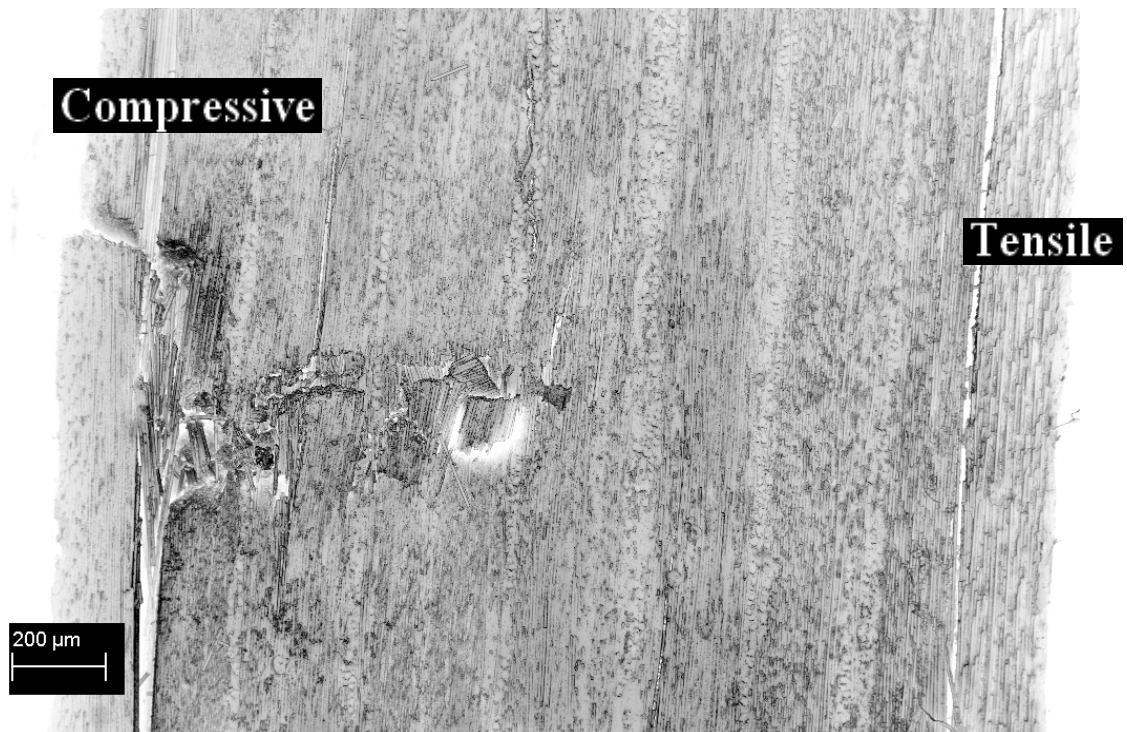
Figure 5.9 SEM micrograph of whole fracture surface of pyrrole (1800 W) treated T700/CNT fiber composite
