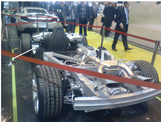
Figure 1.21 McLaren MP4-12C uses lightweight carbon fiber reinforced composite structures (marked with an arrow) for highest power to weight ratio
