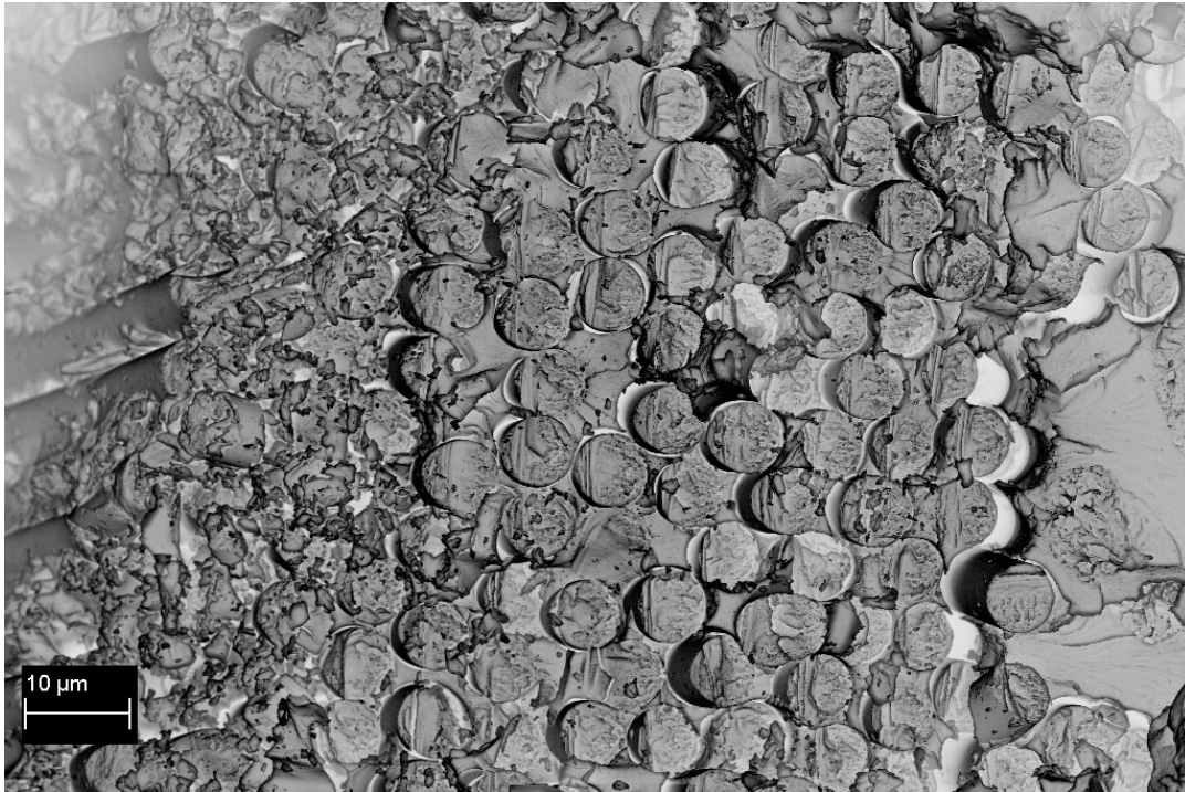
Figure 5.20 SEM micrograph of fiber matrix interface from compression area for pyrrole+dopant (1400 W) treated T700/CNT fiber composite
