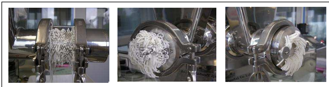
Figure 2- 9: Extrusion of the wet mass for the different extrusion systems: radial, dome, axial.
