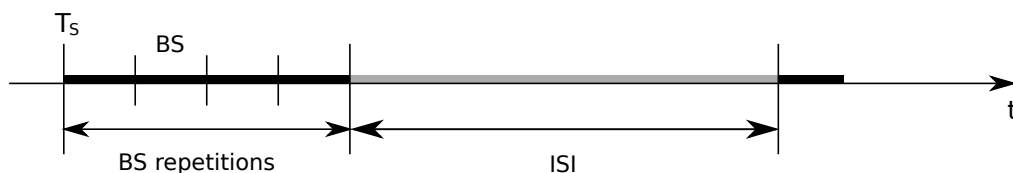
Figure 4.9: Stimulation flow and stimulus structure. A number of repetition of the Base Stimulus followed by an Inter-Stimulus Interval constitutes a elementary stimulus “epoch”.
