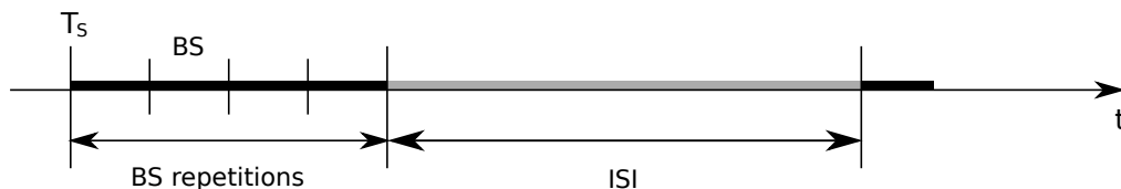
Figure 4.9: Stimulation flow and stimulus structure. A number of repetition of the Base Stimulus followed by an Inter-Stimulus Interval constitutes a elementary stimulus “epoch”.
