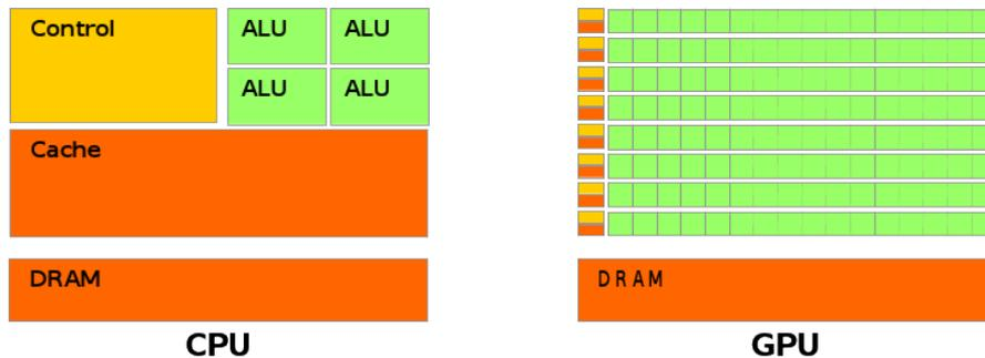
FIGURE 1.4 – Comparaison CPU-GPU
