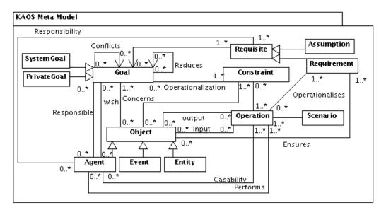
Figure 4.6: KAOS Meta Model adapted from [Dardenne et al., 1993, Heaven et al., 2004]
