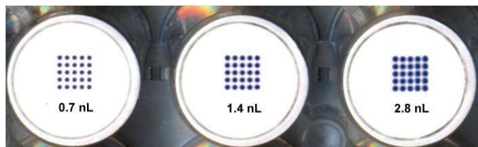
Supplementary Figure 2 | Effect of drop volume on probe density
