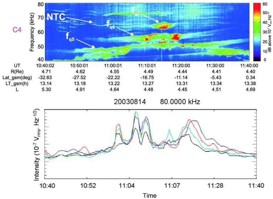
**Fig. 9** (Top) Dynamic time electric field spectrogram of C4 for the 14 August 2003 event. Geomagnetic equator is crossed at about 11:15 UT (latitude is not expressed in SM coordinate system). NTC elements (electromagnetic waves) and a local emission (electrostatic Bernstein mode) are pointed with *arrows*. (Bottom) Compared intensity variations at a given frequency with *colour codes* and constellation configuration as for the event shown in Fig. 8
