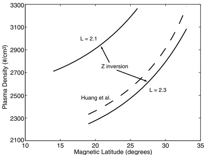
**Fig. 15** Plots of electron density versus *MLAT* at  $L = 2.1$  and 2.3, inferred from the upward propagating Z-mode signals illustrated in Figs. 14a–b and identified as component D in Figs. 14c–d. The *dashed curve* is for  $L = 2.3$  from the Huang et al. (2004) model for a different date. That model is based upon inversion of free-space mode echoes that propagated to RPI along multiple field-aligned paths. (Adapted from Carpenter et al. 2003)
