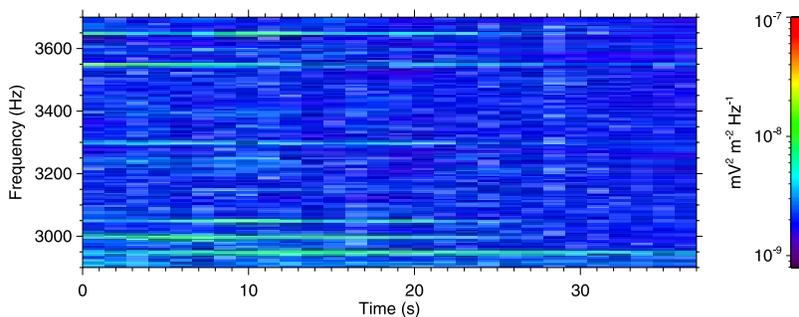
**Figure 1.** An example of frequency-time spectrogram of power spectral density of electric field fluctuations corresponding to one of the identified events. The data were recorded on 21 September 2006 between 10:06:02 and 10:06:39 UT. The lines occur at exact multiples of 50 Hz.
