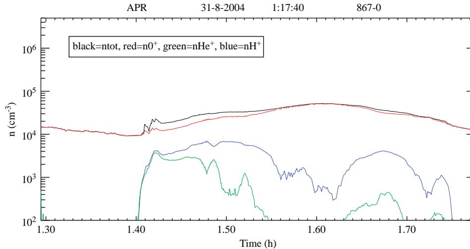
Fig. 4. Measurements of ion density onboard DEMETER on 31 August 2004 (black line) total number density, (red line) number density of  $O^+$  ions, (blue line) number density of  $H^+$  ions, (green line) number density of  $He^+$  ions. Time is given on the bottom in hours from the beginning of the day.
