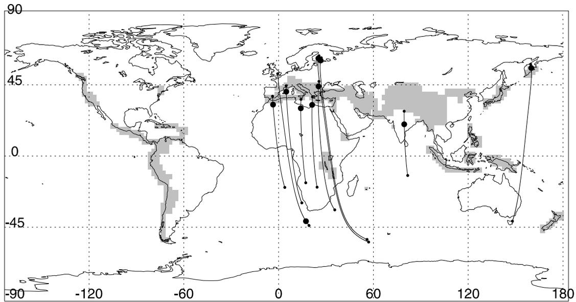
**Figure 2.** Geographic locations of observed PLHR with mutual distance of lines 50/100 Hz (large points). Magnetic field lines and footprints of the points of observations (thin lines and small points). Seismic zones with permanently active burst-mode coverage are shown by gray shading; the operational-phase burst-mode regions (approximately 20% of the burst-mode data volume) are not shown since their positions vary during the time interval analyzed in this study.
