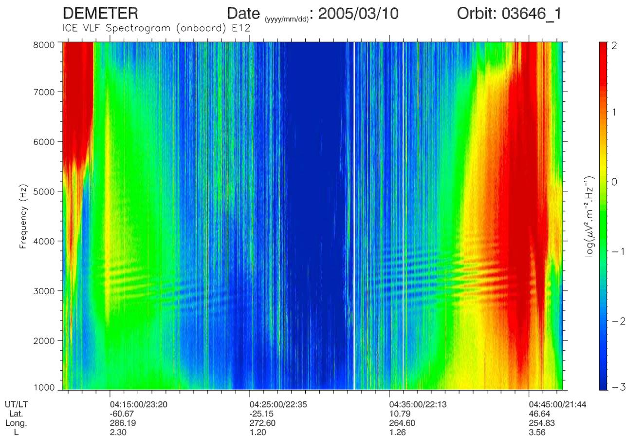
**Figure 1.** An example of a frequency-time spectrogram of a single half-orbit used for the identification of MLR events. Two MLR events at frequencies between about 2.5 and 4 kHz can be clearly seen, located in magnetically conjugate regions.
