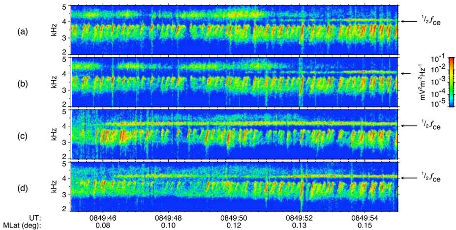
**Fig. 21** Detailed time–frequency power spectrograms of electric field fluctuations in the source region recorded by the WBD instruments onboard the four CLUSTER spacecraft on 18 April 2002. Panels (a)–(d) show data from C1–C4, respectively. *Arrows* indicate local  $\frac{1}{2} f_{ce}$  for each spacecraft. *MLAT* is given on the bottom for C1. Radial distance is  $4.4 R_E$ , and *MLT* is 21:01 during this interval. (Adapted from Santolík and Gurnett 2003)
