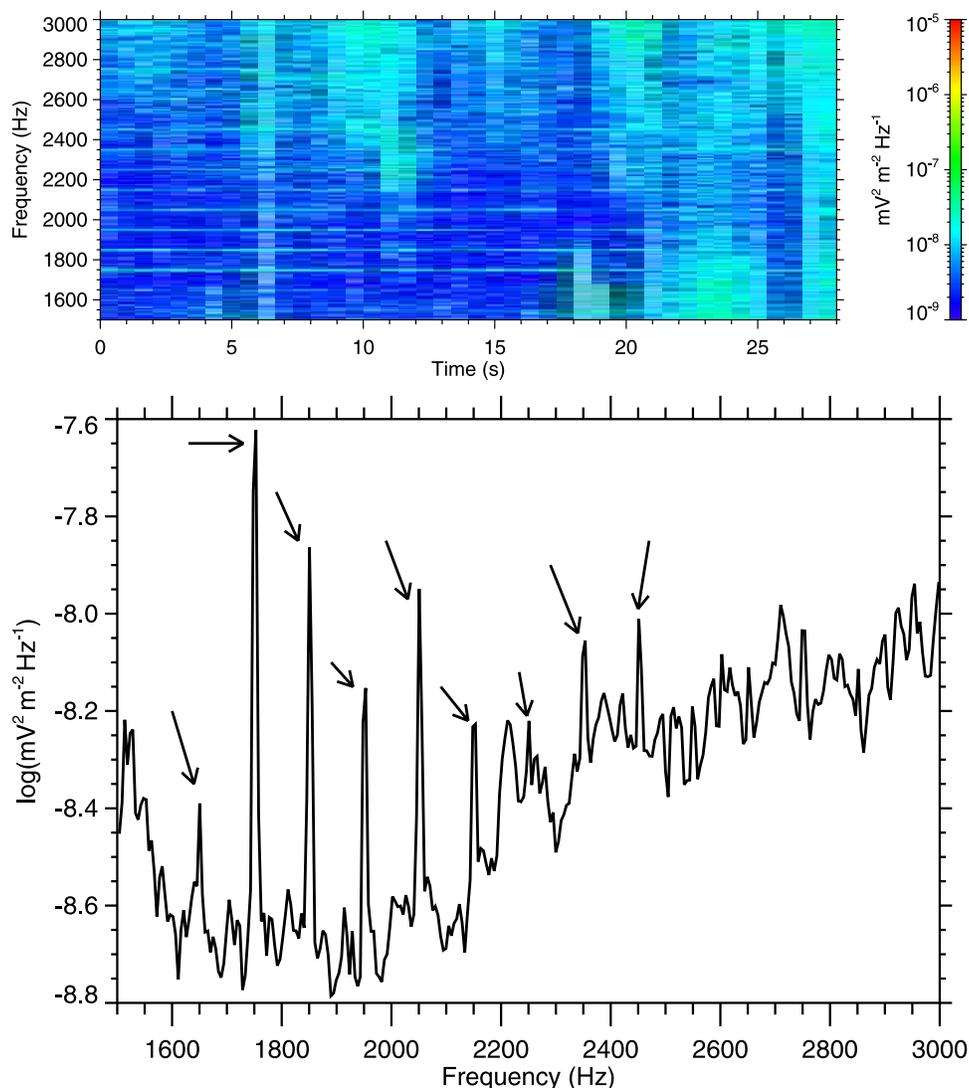
**Figure 2.** Top: An example of frequency-time spectrogram of electric field fluctuations corresponding to one of the analyzed PLHR events with 50/100 Hz spacing. The data were recorded on 25 March 2006 from 1913:32 UT when the spacecraft was flying over Finland. Bottom: Power spectrum of the first 18 s of data, with the most important peaks marked by arrows.
