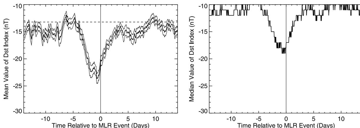
**Figure 8.** (left) Mean value of Dst index as a function of time relative to the time of the MLR event (bold) and standard deviation of the mean value (thin). (right) Median value of Dst index as a function of time relative to the time of the MLR event.
