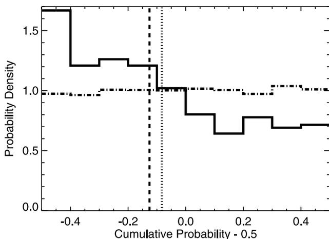
**Figure 2.** (solid line) Distribution of all the cumulative probabilities that contribute to the observed decrease of wave intensity. Mean/median value is plotted by a dotted/dashed line, respectively. (dash-dotted line) Distribution of cumulative probabilities in all bins, but the one wherein the effect is observed.
