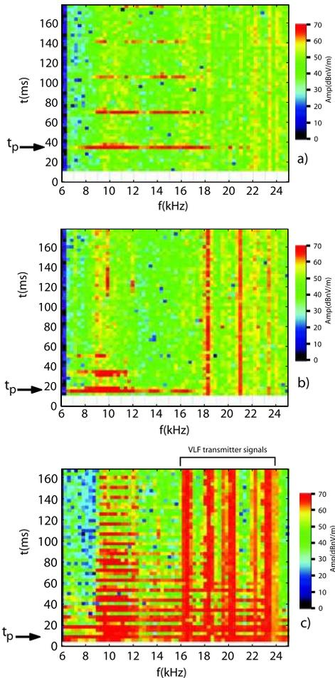
the angle  $\phi$  was near a local minimum of order  $10^\circ$ , WM echoes were observed to repeat at multiples of  $t_p$  up to 15 or more. The data indicate that WM echo detection near 10 kHz was largely confined to a region of radius  $\sim 300$  m around the field line of excitation, and that the peak excitation of the protons occurred as a transient event at the beginning of each radio frequency (*rf*) pulse.
