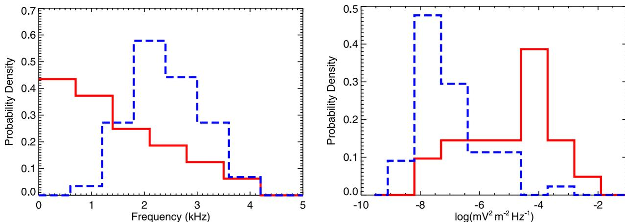
**Figure 5.** Left: Histograms of central frequencies of PLHR events (dashed line) and MLR events (solid line). Right: Histograms of peak intensities of PLHR events (dashed line) and MLR events (solid line).
