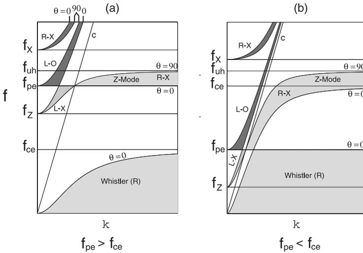
**Fig. 12** Dispersion diagrams for waves in a cold plasma illustrating two conditions on the ratio of electron plasma frequency to electron gyrofrequency: (a)  $f_{pe} > f_{ce}$  and (b)  $f_{pe} < f_{ce}$ . (Adapted from Goertz and Strangeway 1995)
