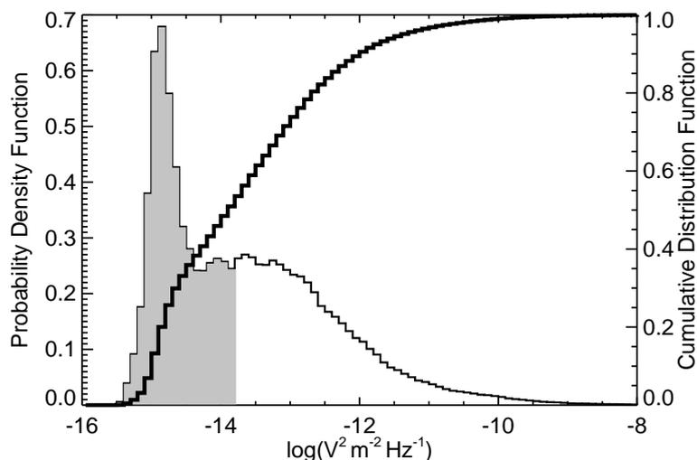
**Figure 1.** Probability density function of the measured power spectral density of electric field fluctuations (thin line) and corresponding cumulative distribution function (thick line). The area corresponding to the values lower than the median value (about  $-13.8 \log(\text{V}^2 \text{ m}^{-2} \text{ Hz}^{-1})$ ) is shaded.
