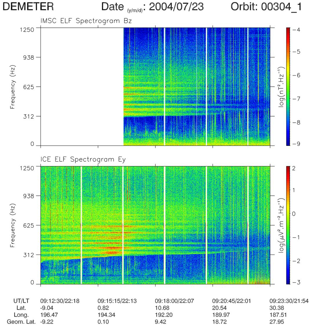
**Fig. 1.** Spectrograms of the magnetic component  $B_x$  (top panel) and  $E_y$  (bottom panel) recorded on 23 July 2004 (event 1). The intensity of the emissions is color-coded according to the color scale on the right. The vertical white lines indicate a change in the mode of the experiment.
