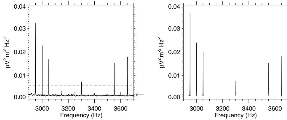
**Figure 2.** (left) Power spectrum corresponding to the event from Figure 1 used for the peak identification procedure. The mean value is marked by an arrow, and the minimum peak value (see text) is plotted by a dashed line. (right) Gaussian fits corresponding to the identified peaks in power spectrum.
