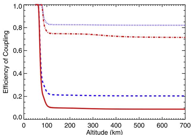
**Figure 11.** Efficiency of coupling for the frequency of wave 2.5 kHz as a function of the altitude for nighttime Finland region (dotted line), nighttime Japan region (dash-dotted line), daytime Finland region (dashed line), and daytime Japan region (solid line).
