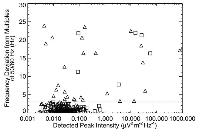
**Figure 9.** Frequency deviation from multiples of power system frequency as a function of the detected peak intensity. The lines forming events with frequency spacing 50/100 Hz are plotted by triangles, and the lines forming events with frequency spacing 60/120 Hz are plotted by squares.
