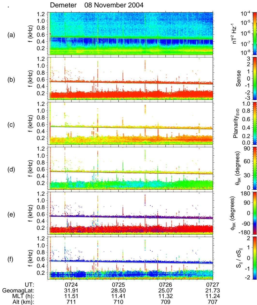
**Fig. 9.** Wave analysis of the event 2. (a) spectrogram of one magnetic component, (b) sense of polarization, (c) planarity, (d) and (e) polar and azimuthal angles of the wave vector with the Earth’s magnetic field  $B_0$ , (f) projection of the Poynting vector onto  $B_0$  (see text for explanation). The geophysical parameters at the bottom are the Universal Time (UT), the geomagnetic latitude, the Magnetic Local Time (MLT) and the altitude.
