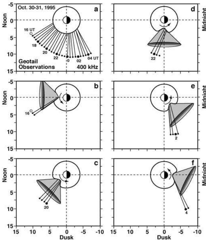
**Fig. 4** Direction finding measurement (a) from Hashimoto et al. (1999) of KC at 400 kHz are reinterpreted as being completely consistent with respect to the source of KC emitted from a corotating plasmaspheric notch (b)–(f). (Adapted from Green et al. 2002)
