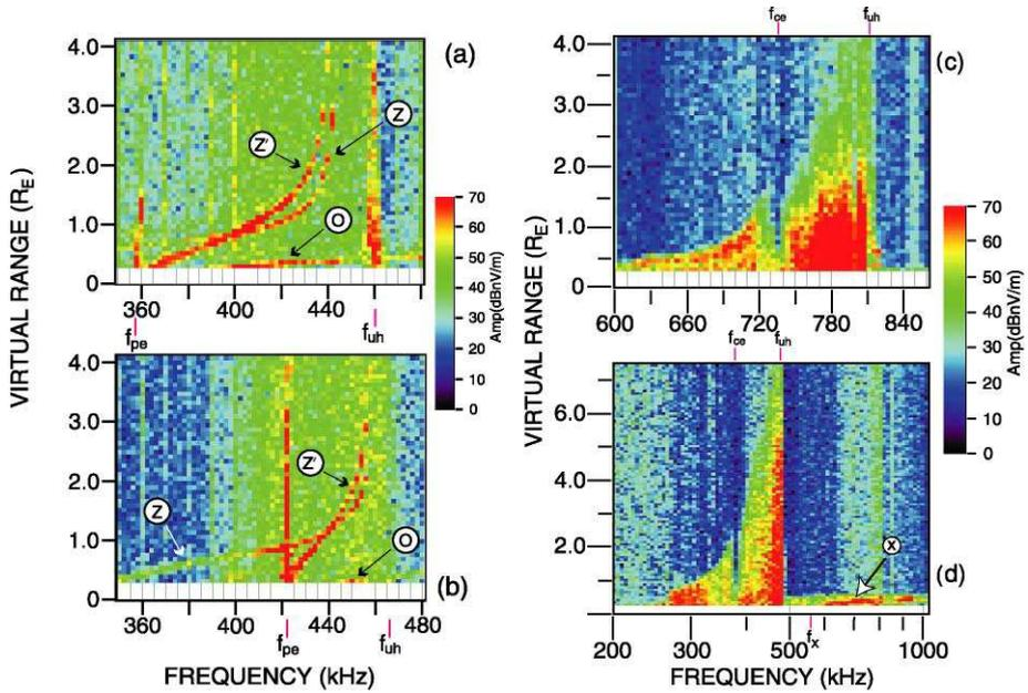
**Fig. 17** (a)–(b) RPI plasmagrams illustrating Earthward propagating discrete Z and Z' echoes seen against a background of diffuse Z-mode noise. (c)–(d) RPI plasmagrams typical of low altitude polar regions showing diffuse Z-mode echo activity useful for determining  $f_{ce}$  and  $f_{pe}$ . (Adapted from Carpenter et al. 2003)
