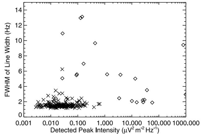
**Figure 8.** FWHM of frequency ranges of individual lines forming the PLHR events as a function of the peak intensity. The events with frequencies corresponding to the multiples of the power system frequency are plotted by crosses, and the events with frequencies not corresponding to these multiples are shown by diamonds.
