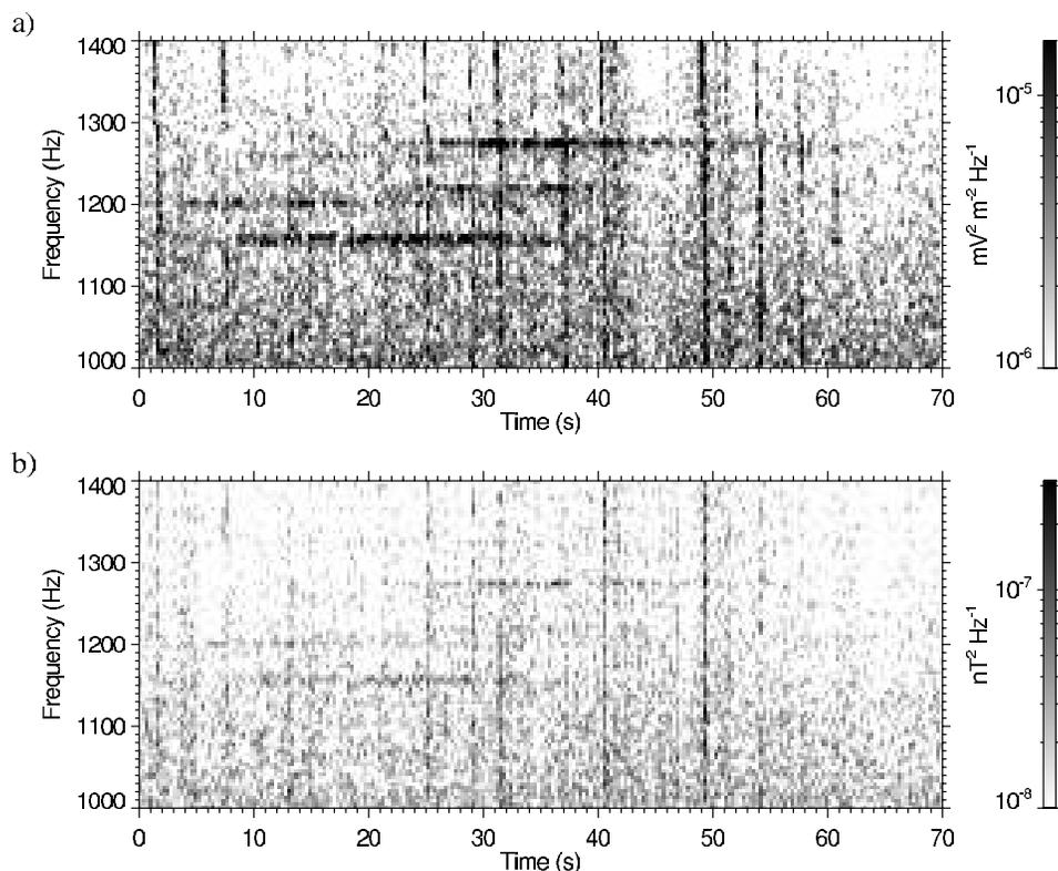
**Figure 1.** An example of (a) frequency-time spectrogram of the electric and (b) magnetic field fluctuations corresponding to one of the analyzed events. The data were recorded on 11 November 2004, after 1400:05 UT, when the spacecraft overflew Philippines; the frequency separation of the spectral lines is 60 Hz.
