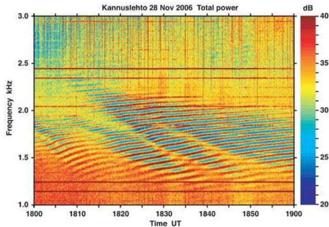
**Figure 1.** Spectrogram of the signal received at Kannuslehto between 18.00 and 19.00 UT. The frequency range is between 1 and 3 kHz. The signal intensity is color coded according to the scale on the right. The horizontal lines observed just above 1 kHz and between 2 and 3 kHz are the PLHR which are at exact harmonics of 50 Hz. MLR with drifting frequencies are observed between 1.2 and 2.4 kHz.
