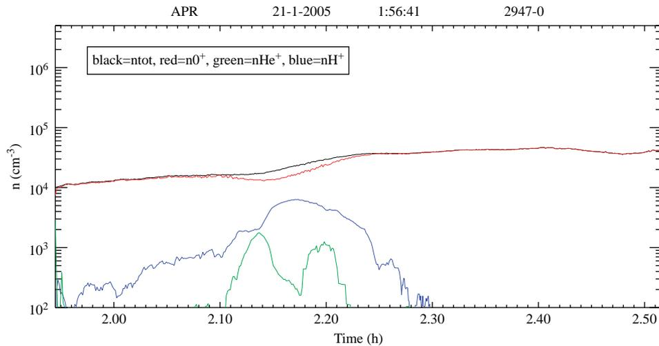
Fig. 8. Measurements of ion density onboard DEMETER on 21 January 2005: (black line) total number density, (red line) number density of  $O^+$  ions, (blue line) number density of  $H^+$  ions, (green line) number density of  $He^+$  ions. Time is given on the bottom in hours from the beginning of the day.
