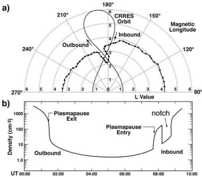
**Fig. 5** (a) A typical orbit of the CRRES spacecraft in magnetic longitude and  $L$  value plotted over a typical plasmaspheric notch. (b) Approximate variation in density that would be observed assuming that a notch structure like this would exist at the time of CRRES
