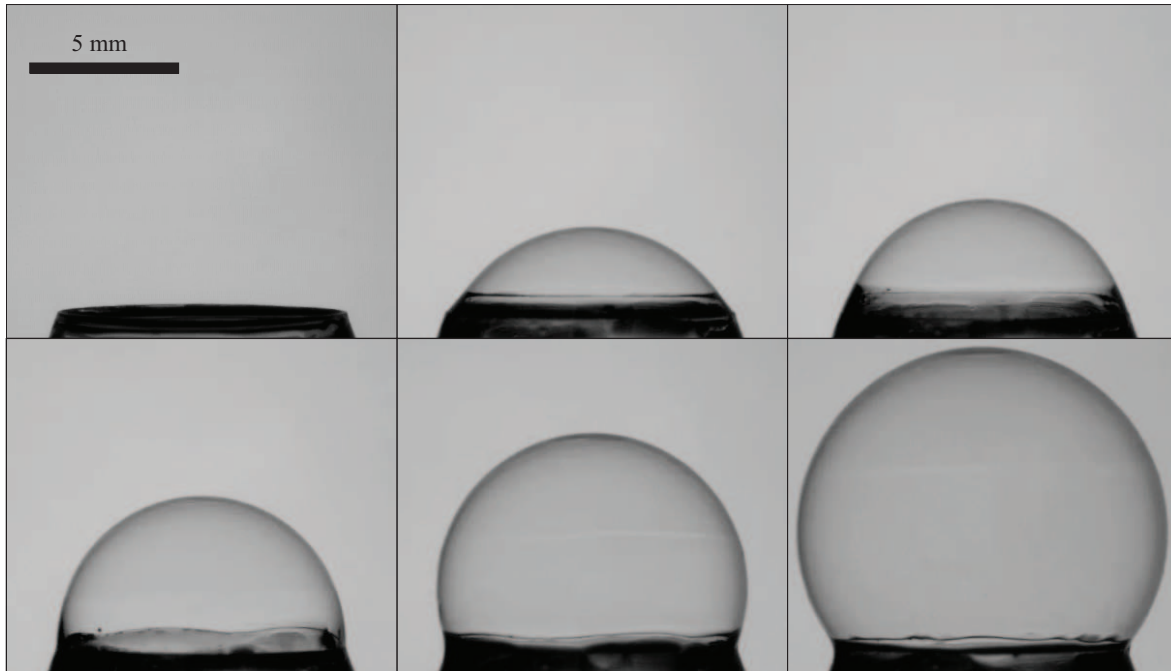
Figure A.3: Film bulging when injecting a constant air flow-rate – The film geometry is later fitted by an circle arc (see text) [ \Phi = 25 mL/s].
