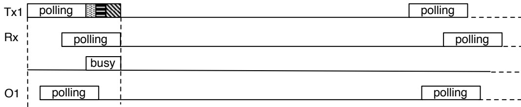
FIGURE 4.2 – X-MAC protocol, global buffer size B = 1 . Overhearing situations for Case 1.
