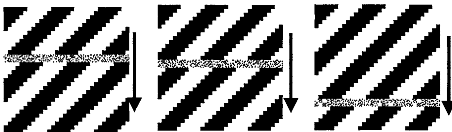
FIGURE 6b The sliding grating scheme. A narrow window of updating pixels slides down the displayed image to change the image.
