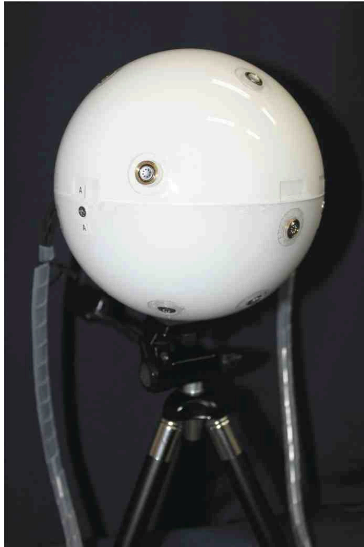
Figure 6.1 The fabricated 12-element icosahedral microphone array with the microphones fixed on a spherical shell rigid mount. The diameter is 15cm.
