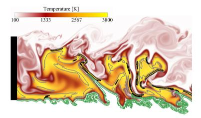
Figure 3.29: Close-up view of the flame stabilization zone behind the splitter. Temperature field with superimposed iso-contours of density gradient (green= $4 \ 10^7 \ \text{kg/m}^4$ ) and heat-release rate (grey= $10^{12} \ \text{W/m}^3$ , black= $10^{13} \ \text{W/m}^3$ ).
