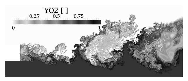
Figure 3.10: Non-reacting flow:  $O_2$  mass fraction field, showing the rapid mixing of the two streams by a large range of vortical structures.
