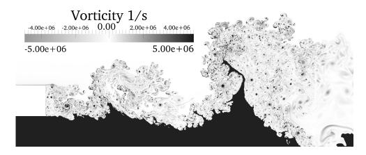
Figure 3.17: Non-reacting flow: vorticity field superimposed on the high-density region (fluid regions with a density that is higher than  $\rho_{0.5} = 0.5 \ (\rho_{H_2}^{inj} + \rho_{O_2}^{inj})$  are painted in black.).
