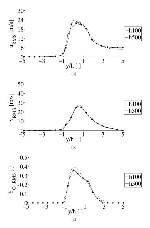
Figure 3.27: RMS profiles, at x = 5h for the h100 and h500 meshes, of (a) axial velocity, (b) transverse velocity and (c)  $O_2$  mass fraction.
