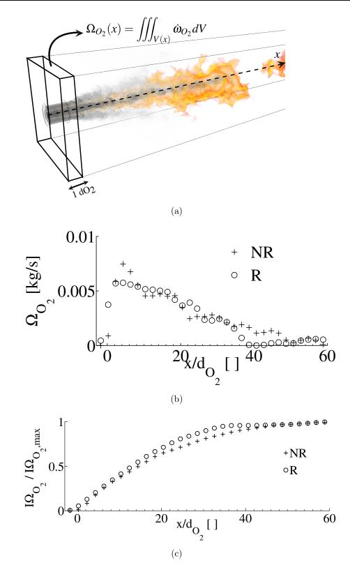
Figure 4.17: (a) Definition and (b) distribution of the integrated consumption rate of oxygen  $\dot{\Omega}_{O_2}$ . (c) Normalized and cumulated consumption rate of oxygen  $I\dot{\Omega}_{O_2}/I\dot{\Omega}_{O_2,max}$  (defined in Eq. 4.13)
