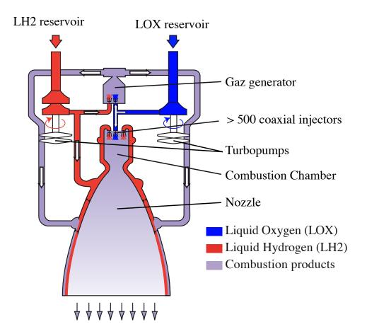
Figure 1.3: Operating principle of the Vulcain 2 engine [Snecma 2011].
