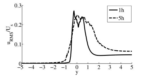
Figure 3.23: Non-reacting flow: transverse cuts of the RMS axial velocity normalized by the velocity difference  $U_s = U_{H_2}^{inj} - U_{O_2}^{inj}$  at x=1h and x=5h.
