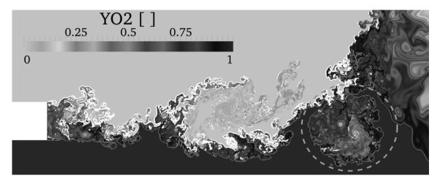
Figure 3.18: Non-reacting flow:  $O_2$  mass fraction, along with a grey isocontour of middensity ( $\rho = 637 \text{ kg.m}^{-3}$ ) and a white isocontour of high scalar dissipation rate ( $\chi = 5 \ 10^3 \text{ s}^{-1}$ ). The dash circle shows a region of low scalar dissipation rate where mixing has already occurred.
