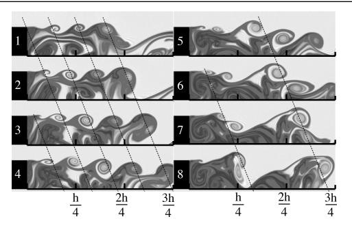
Figure 3.9: Non-reacting flow: oxygen mass fraction field at the  $H_2$  corner of the lip, at successive instants. The time interval between frames is 10  $\mu$ s
