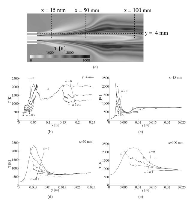
Figure 4.13: NR configuration: comparison between H<sub>2</sub> CARS measurements and conditional temperatures  $T_{\alpha}$ , defined in Eq. 4.11.  $\circ$ : CARS measurements from [Habiballah *et al.* 2006] and [Zurbach 2006]. (a) positions of the cuts (b) y = 4 mm, (c) x = 15 mm, (d) x = 50 mm, (e) x = 100 mm.
