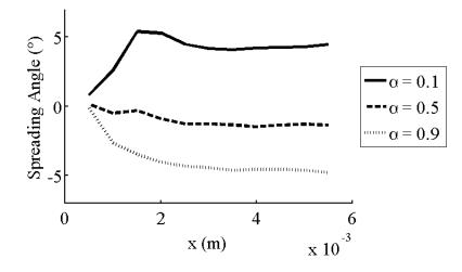
Figure 3.21: Non-reacting flow: spreading angles  $\theta_{\rho,\alpha}$ .
