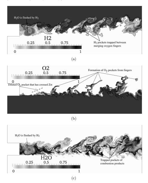
Figure 3.33: Reacting flow: instantaneous fields of (a) hydrogen (b) oxygen and (c) water mass fraction, with superimposed stoichiometric mixture fraction isoline (black). The dash line in (b) shows the location of the 1D cut that is used in Fig. 3.34.
