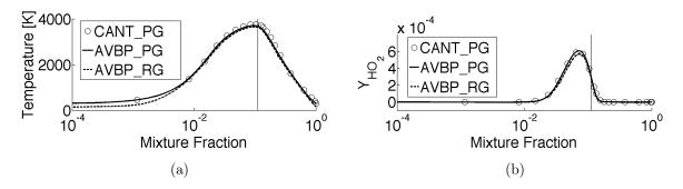
Figure 3.6: Comparison of flame structure versus mixture fraction between AVBP and CANTERA. (a) temperature and (b)  $HO_2$  mass fraction. The vertical bar indicates the stoichiometric mixture fraction.
