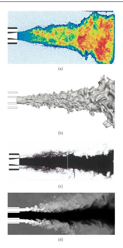
Figure 4.7: Qualitative comparison between instantaneous experimental ((a) and (c)) and numerical ((b) and (d)) visualizations of the reacting flow: (a) OH<sup>\*</sup> emission (b) T = 1500 K iso-surface (c) shadowgraph (d) mixture fraction between 0 (black) and 1 (white).
