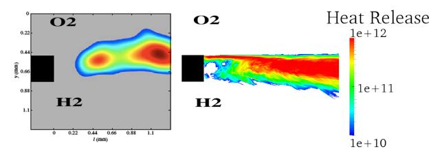
Figure 3.40: Comparison between experimental signal of OH PLIF [Singla *et al.* 2007] at transcritical conditions and time averaged heat release rate in the current simulation (the numerical visualization is upside down to compare with experimental visualization)
