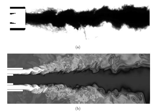
Figure 4.15: Qualitative comparison for the R configuration, between an instantaneous (a) experimental shadowgraph and (b) a mixture fraction field between 0 (black) and 1 (white).
