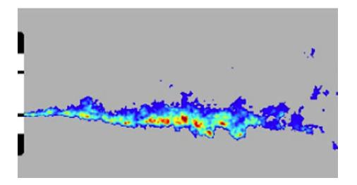
Figure 1.8: OH PLIF image of a  $LOx/GH_2$  cryogenic flame [Singla *et al.* 2007].
