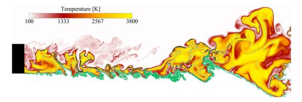
Figure 3.28: Temperature field with superimposed density gradient (green) and heat-release (black: max heat release rate of case AVBP\_RG (= $10^{13}$  W/m<sup>3</sup>); grey: 10 % of case AVBP\_RG (= $10^{12}$  W/m<sup>3</sup>).
