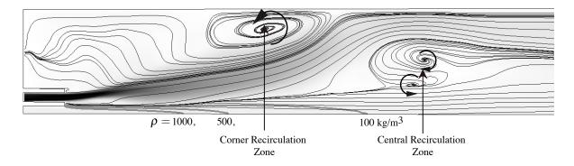
Figure 4.10: Cut of the average velocity magnitude (white = 0 m/s; black = 200 m/s) with superimposed streamlines in black and density iso-contours in grey ( $\rho$ =100, 500, 1000 kg/m<sup>3</sup>), obtained with the h5 mesh.
