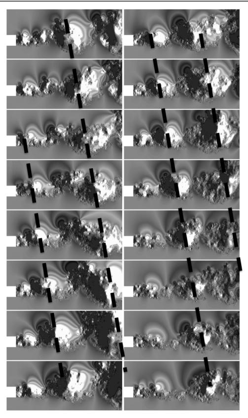
Figure 3.11: Non-reacting flow: temporal evolution of the transverse velocity field. The time interval between two snapshots is  $\tau_{conv}$
