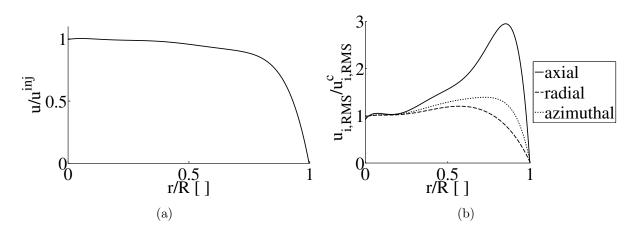
Figure 4.5: Turbulence injection profiles: a) mean axial velocity and b) Root Mean Square velocity fluctuations. The superscript c refers to the centerline value.
