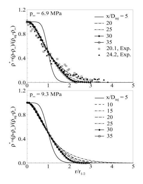
Figure 1.11: Radial distributions of normalized density at different axial locations ( $T_{\infty} = 300 \text{ K}, u_{inj} = 15 \text{ m/s}, T_{inj} = 120 \text{ K}, D_{inj} = 254 \text{ }\mu\text{m}$ ) [Zong & Yang 2006]
