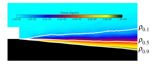
Figure 3.20: Non-reacting flow: average density field
