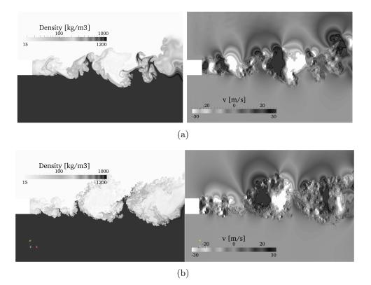
Figure 3.25: Instantaneous snapshots of the transverse velocity and the density for the (a) h100 and (b) h500 meshes.
