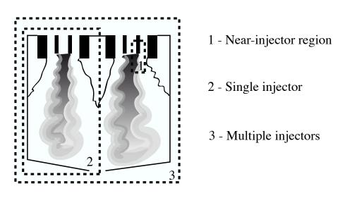
Figure 1.14: Schematic of a LRE combustion chamber, showing the different levels of study considered in the present thesis work.
