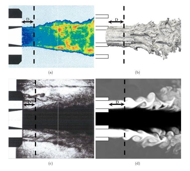
Figure 4.9: Qualitative comparison between instantaneous experimental ((a) and (c)) and numerical ((b) and (d)) visualizations of the near-injector region of the reacting flow: (a) OH<sup>\*</sup> emission (b) T = 1500 K iso-surface (c) shadowgraph (d) mixture fraction (black=0; white=1).
