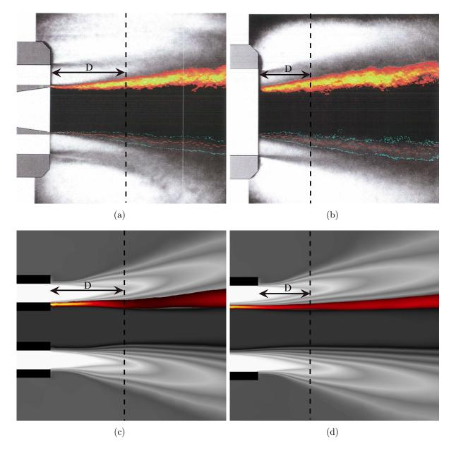
Figure 4.16: Time-averaged results. NR configuration (left) and R configuration (right): (a) and (b) are experimental shadowgraphs and Abel-transformed  $OH^*$  emissions, (c) and (d) are mixture fraction fields (black=0; white=1) and temperature fields (black=1000 K; yellow=3000 K).
