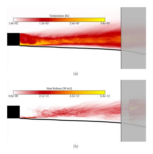
Figure 3.37: Average fields for the reacting flow. (a) Temperature. (b) Heat release rate. Black iso-contour:  $\rho_{0.9}$ .
