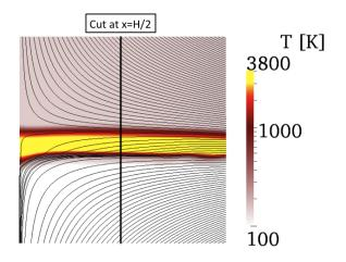
Figure 3.5: Strained diffusion flame computed in AVBP: streamlines superimposed on the temperature field. Thermodynamic conditions correspond to the splitter case: hydrogen at 150 K from the top, oxygen at 100 K from the bottom and ambient pressure is 10 MPa.
