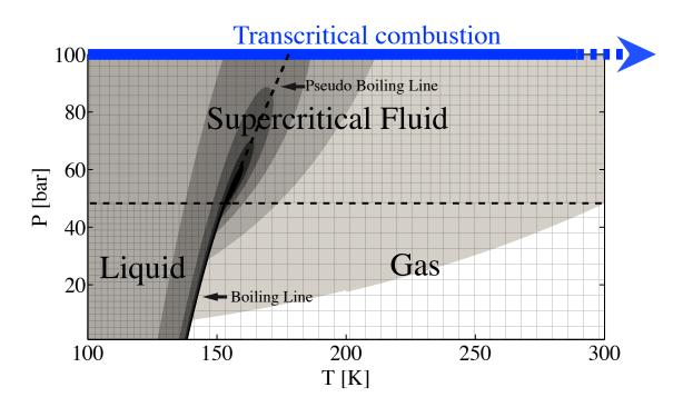
Figure 1.5: Heat capacity isocontours computed with the Soave-Redlich-Kwong equation of state (see Eq. 2.44): white  $= 10^3 \text{ J/K/kg}$ ; black $= 10^4 \text{ J/K/kg}$ .
