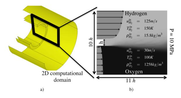
Figure 3.1: a) Typical coaxial injector of a LRE. b) Boundary conditions for the 2D computational domain
