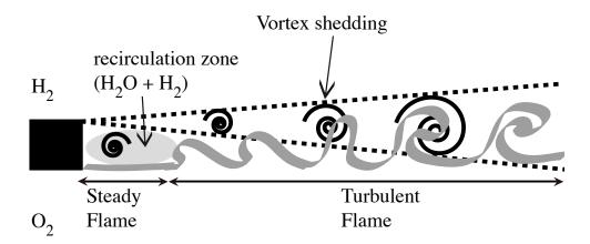
Figure 3.30: The flame/vortex interaction separates the flame into 2 zones, a near-injector steady diffusion flame between  $O_2$  and a mixture of  $H_2$  and  $H_2O$ , and a turbulent flame developing further downstream.
