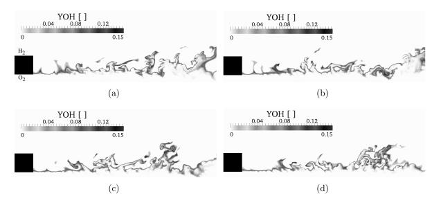
Figure 3.38: OH mass-fraction fields at four instants. Liquid oxygen and gaseous hydrogen are injected below and above the step, respectively.
