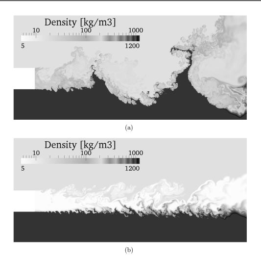
Figure 3.31: Comparison of the density fields between a) the non-reacting flow and b) the reacting flow
