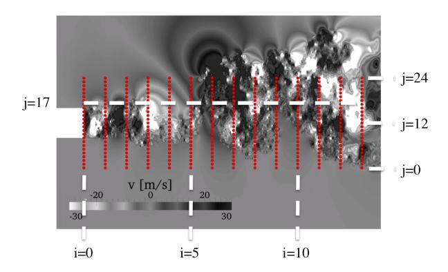
Figure 3.2: Probes located in the mixing layer.
