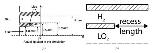
Figure 4.2: Geometry of the coaxial injectors: a) dimensions and b) recess length.
