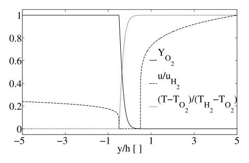
Figure 3.3: Transverse cut through the initial solution of the cold flow, downstream the lip.
