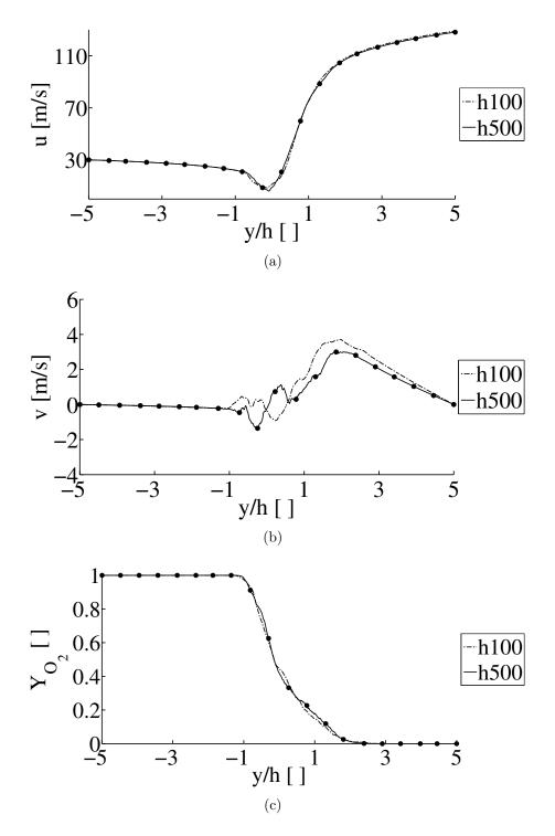
Figure 3.26: Mean profiles, at x = 5h for the h100 and h500 meshes of (a) axial velocity, (b) transverse velocity and (c)  $O_2$  mass fraction
