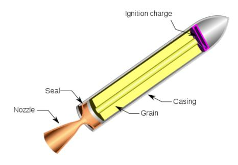
Figure 1.2: Components of a booster.
