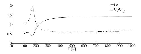
Figure 2.2: Evolution of the Lewis number and normalized heat capacity with temperature.  $C_{p,0} = 1700 \text{ J/K/kg}$ . The peak of  $C_p$  at the pseudo-boiling point creates a local minimum in the Lewis number.
