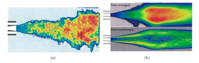
Figure 1.7: Flame shape visualizations using  $OH^*$ , in a coaxial  $LOx/GH_2$  injector [Juniper 2001]: (a) instantaneous image, (b) top: time-averaged image; bottom: Abel-transformed image. The pressure is 7 MPa.
