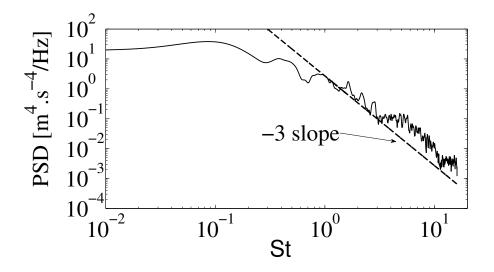
Figure 3.16: Non-reacting flow: power spectrum density of the squared transverse velocity at i=10, j=12. Eight Welch averaging windows are used.
