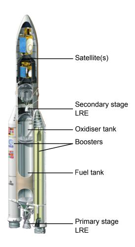
Figure 1.1: The main components of the Ariane 5 european space launcher.
