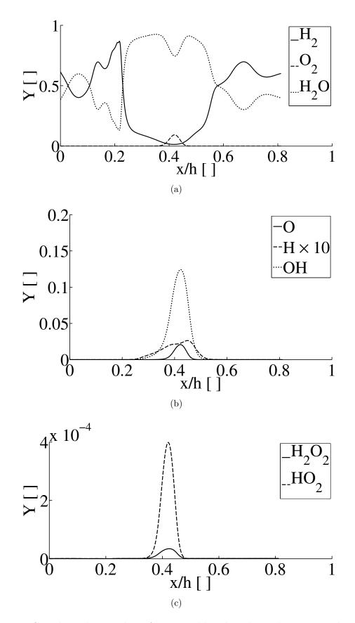
Figure 3.34: Cut through a pocket of oxygen diluted with combustion products. The location of the 1D cut is shown by a dash line in Fig. 3.33(b).
