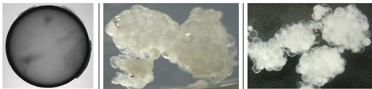
Figure V.13: Picture of a shell, on the left, and pictures of shells agglomerates, obtained during the synthesis of shells with 1% DMPA
