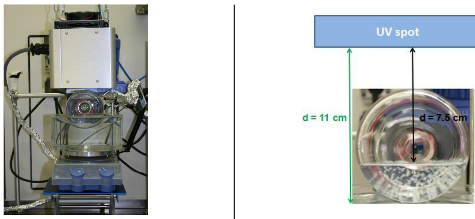
Figure V.19: On the left, picture of the UV spot placed on top of the rotating flask. On the right, illustration of the distance between the UV spot and the flask filled with shells
