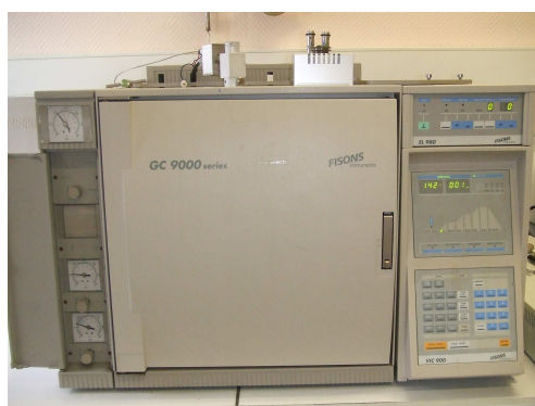
Figure A.1: Gas chromatography GC 9000 series from Fisons Instruments
