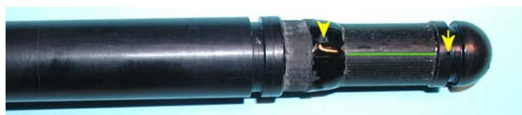
Figure III.1. Head of the 64-element rectal ultrasound applicator (diameter: 14 mm; working frequency: 3.57 MHz). The surface of a single element (20 x 0.6 mm 2 ) is highlighted with the green line. The arrows indicate the opening of the two thin pipes, which ensure the water flow, along the active zone of the transducer and on its rigid backing part.
