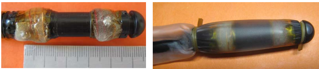
Figure IV.9. Opposed-solenoid RF coil integrated within the phased-array esophageal transducer (without and with the cooling balloon).
