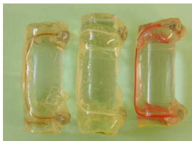
Figure IV.6. Diverse wiring tested in order to define the prototype esophageal coil.
