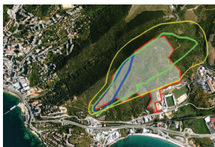
FIGURE 13: Case 1: Simulations results and observations for the Vazzio fire. Blue: simulated fire contour at 15:30 (after 1 h), Green: simulated contour at 18:30, Yellow: Simulated contour at 18:30 (non coupled); Red: final observed contour of the fire.
