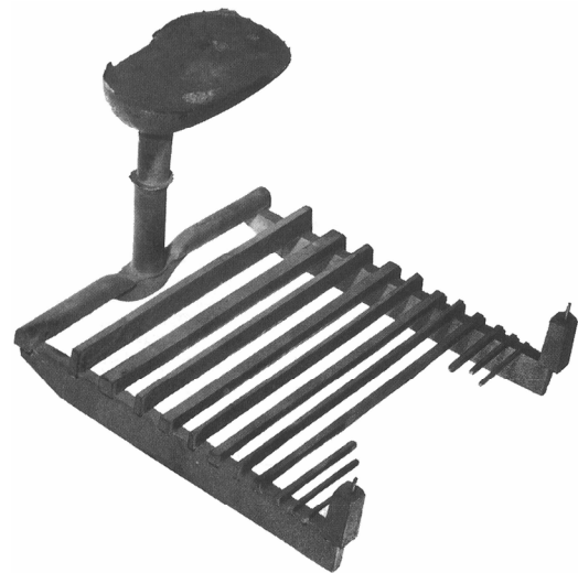
Figure IV-3 - Eprouvette C.T.I.F-Olivier [AYM1996].
