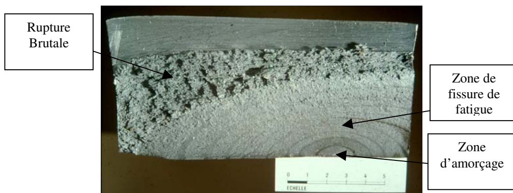
Figure 7 : Faciès de rupture
