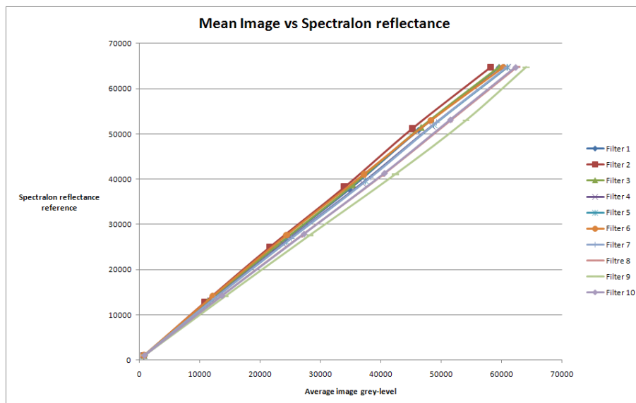
Figure 3.14: Camera linear response.
