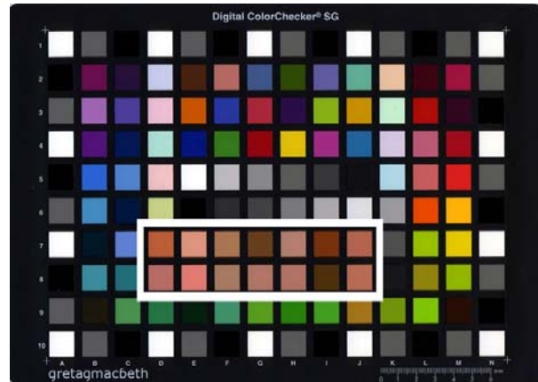
Figure 3.17: Digital ColorChecker ® SG with skin-tone patches highlight.
