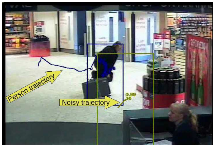
Figure 6.5 – Illustration of a noisy trajectory
