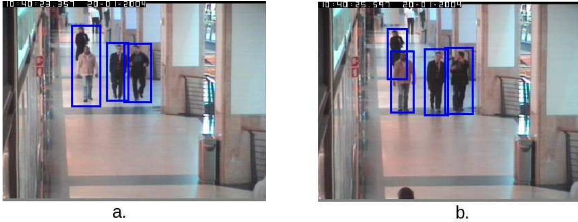
Figure 5.2 – Illustration of the influence of the object detection quality (produced by approach [Corvee and Bremond, 2010]) due to object location : a. Left image : at frame 279, the two persons on the left are wrongly detected because the head of the top person and the foot of the bottom person are considered as belonging to a same person b. Right image : at frame 335, the relative position of these two persons is changed, and they are correctly detected.
