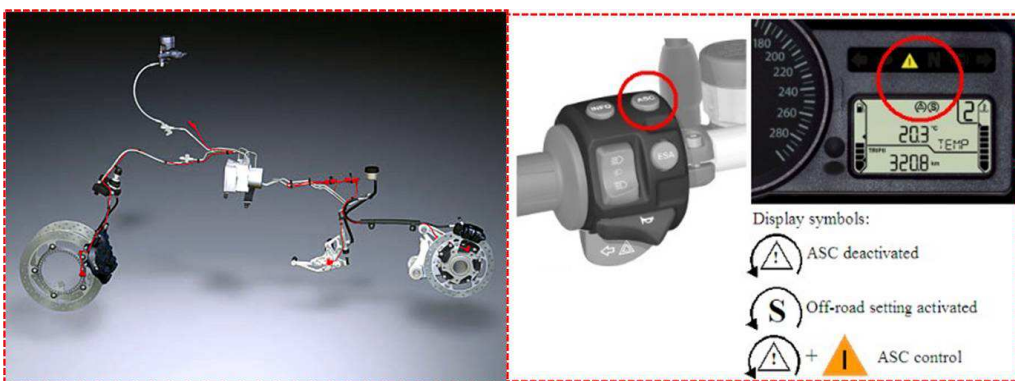
FIGURE 1.4 – Automatic Stability Program (ASC) pour moto
