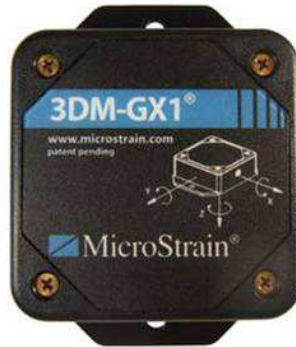
FIGURE 5.17 – Centrale inertielle 3DM-GX1
