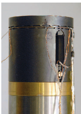
Fig. 1.13. Bending TARSIS device and an example of the force-displacement characteristic of MIT strand at 4.2 K (Courtesy of Nijhuis).
