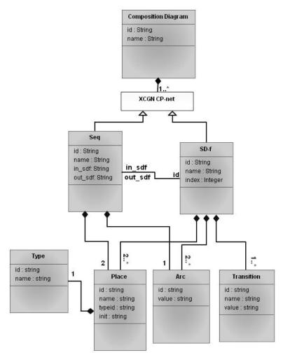
Figure 20: Composition diagram data type
