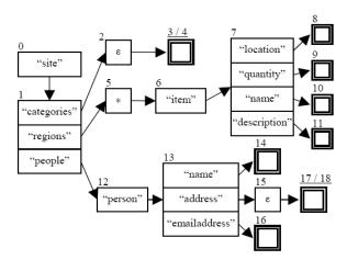
Figure 12: User queries defined with XPath expressions for the required filter and the corresponding NFA
