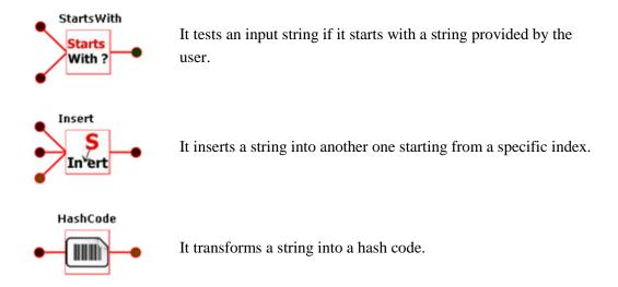
Figure 4: Several sample functions defined in XCDL
