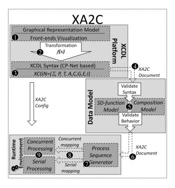
Figure 2: Architecture of the XA2C framework
