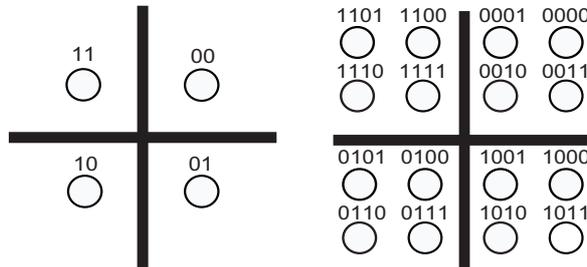
Figure 2.4: 4-QAM (left) and 16-QAM (right)
