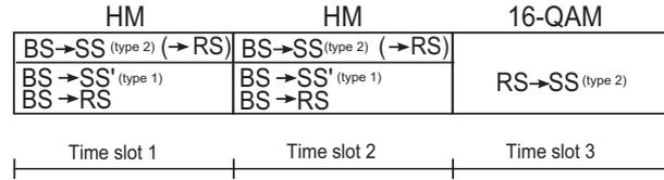
Figure 5.6: Enhanced HM-based adaptive relaying scheme
