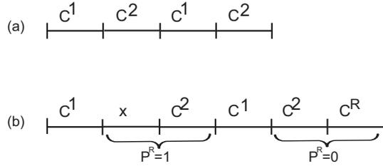
Figure 6.3: (a) Classical TDM scheme and (b) HM-based relaying scheme
