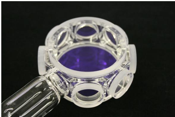
(a) Glass chamber used to create the MOT with multiple input ports.
