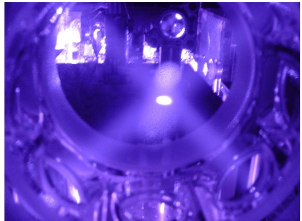
(b) Atoms trapped at the center of the chamber
