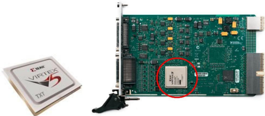
(a) Example Xilinx FPGA before mounting onto a circuit.
