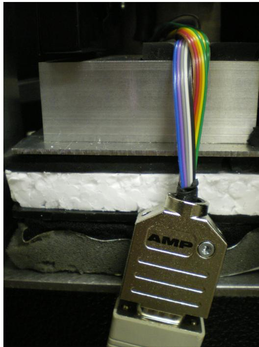
Figure 5.20: Isolation sandwich used to attenuate chopper vibrations, consisting of aluminum, lead, styrofoam, and sorbothane.
