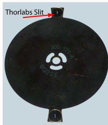
Figure 5.17: Customized disc designed to hold both  $200\ \mu\text{m}$  and  $50\ \mu\text{m}$  Thorlabs slits.
