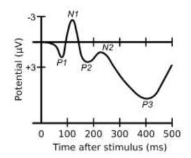
Figure 1.4: An ERP is any measured brain response that is directly the results of thought or perceptron. The wave shows several ERP components, including the N100 and P300 (from Wikipedia).
