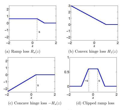
Figure 2.3: Illustration of Ramp loss  $R_s(z) = H_1(z) - H_s(z)$  and the clipped symmetric hinge loss function U(|z|) for unlabeled data.
