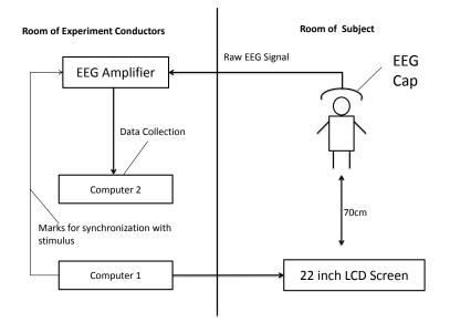
Figure 4.5: Experimental diagram of the emotional BCI system.
