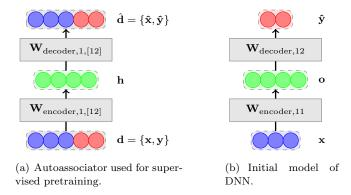
Figure 1.8: A toy example of a supervised pretraining strategy. 1.8(a): an autoassociator learned on input  $\mathbf{d} = \{\mathbf{x}, \mathbf{y}\}$ . 1.8(b): the initial last hidden layer and the initial output layer ( $\mathbf{W}_{encoder,11}$  is the part of  $\mathbf{W}_{encoder}$  that corresponding to input  $\mathbf{x}$ ,  $\mathbf{W}_{decoder,12}$  is the part of  $\mathbf{W}_{decoder}$  that corresponding to output  $\mathbf{y}$ ).
