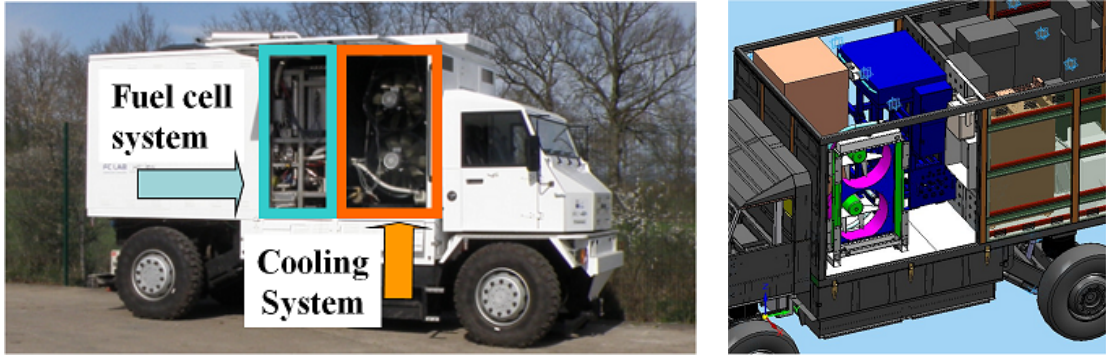
Figure 2.16: Fuel cell system implemented in ECCE
