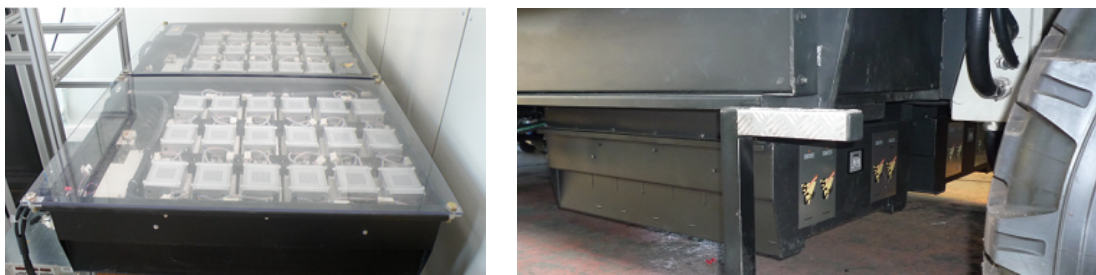
Figure 2.7: SAFT ultracapacitors implemented in ECCE
